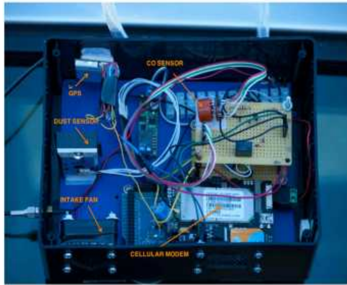
Figure 2.10 Mobile Sensing Box used for Air Pollution Data Collection (MSB) (2007) [24]
