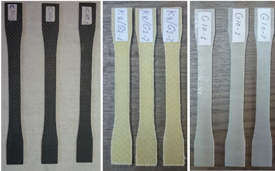
Figure 3.6 Examples of tensile test specimens
