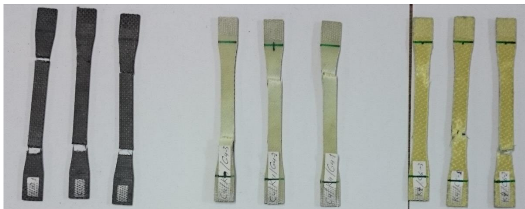
Figure 4.6 Failure specimens of different composite laminates after tensile test.
