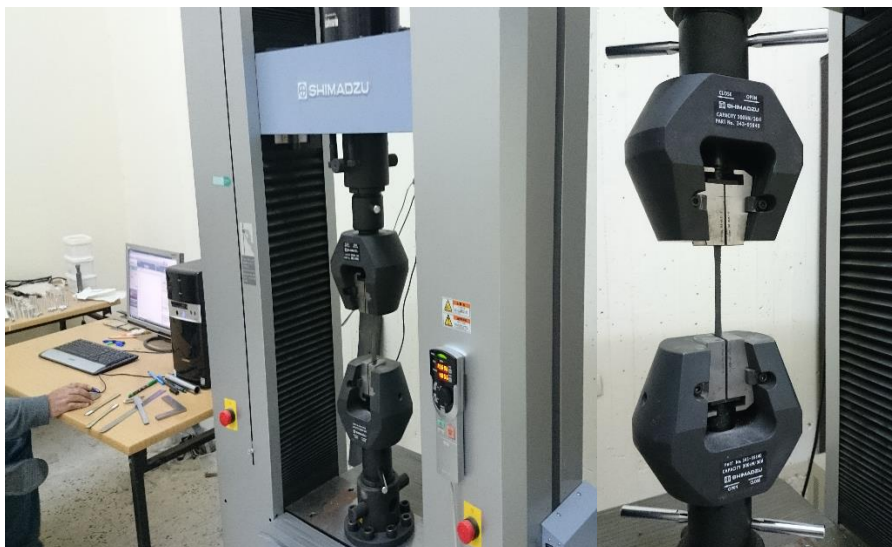
Figure 3.8 Test set-up Shimadzu AG-X series testing machine (tensile test)
