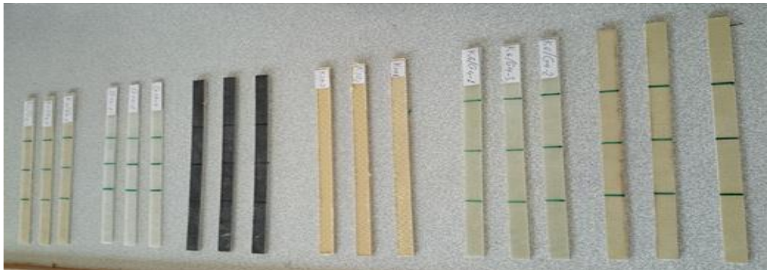
Figure 3.10 Examples of flexural test specimens
