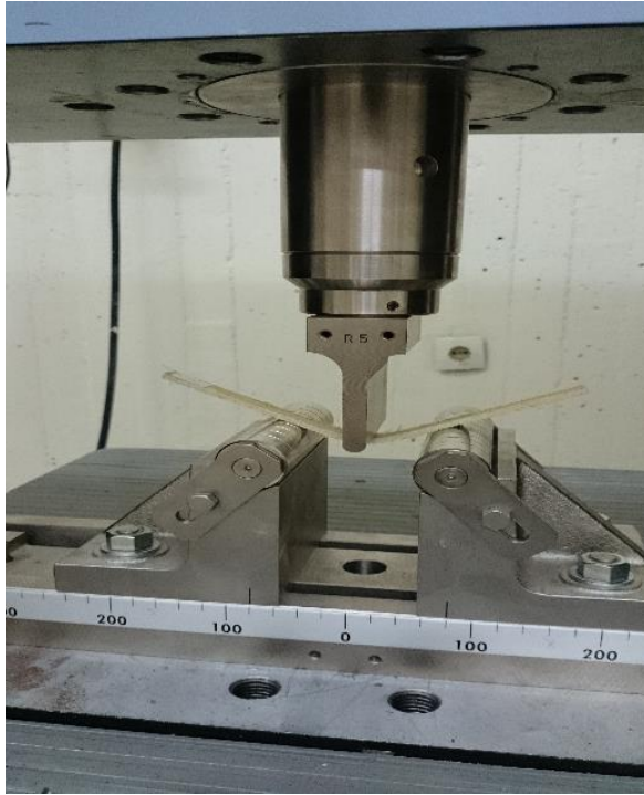
Figure 3.9 Test set-up Shimadzu AG-X series testing machine (flexural test)
