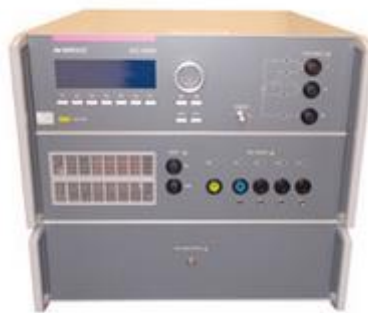
Figure 4.15 Damped oscillatory wave and ringwave simulator
