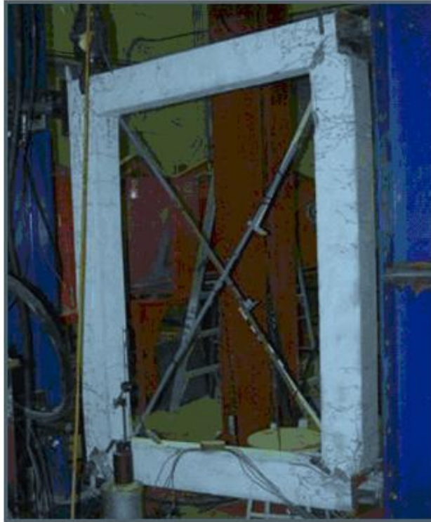
Figure 2.14 Steel-braced reinforced concrete frame (Maheri and Ghaffarzadeh, 2008)
