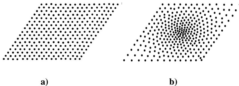
Figure 5.12. The EFGM models for a) regular node distributions, b) irregular node distributions
