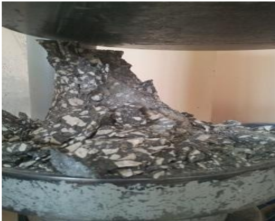
Figure 4.2a Failure mode of SCC specimen without rubber particles under uniaxial compression
