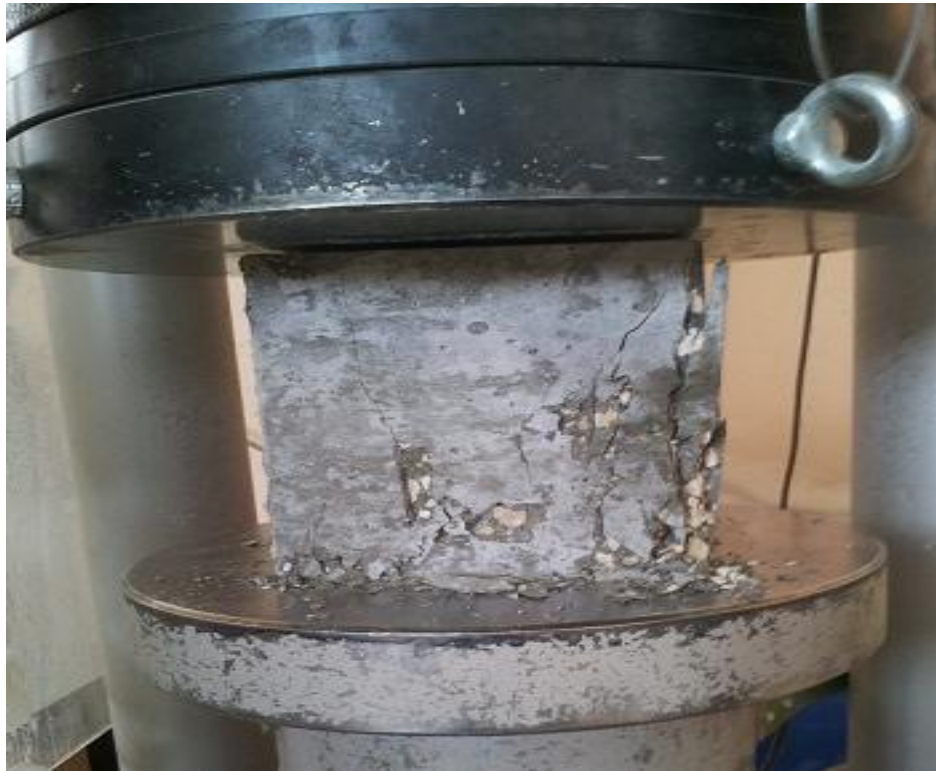
Figure 4.2b Failure mode of SCRC specimen with 40% rubber particles under uniaxial compression.
