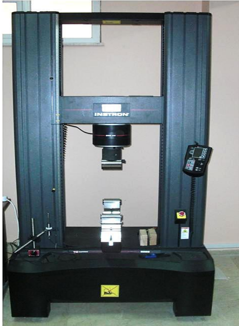
Figure 3.5 Photographic view of universal testing devices and three point flexural testing fixture
