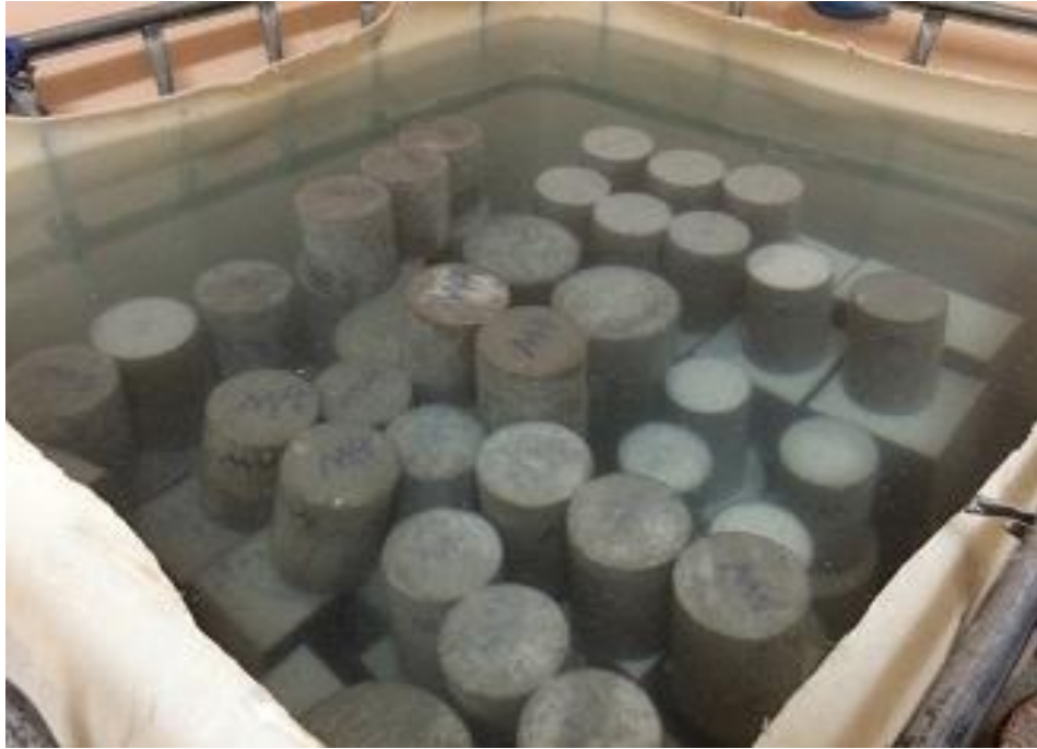
Figure 3.3 Curing of self-compacting rubberized concrete specimens
