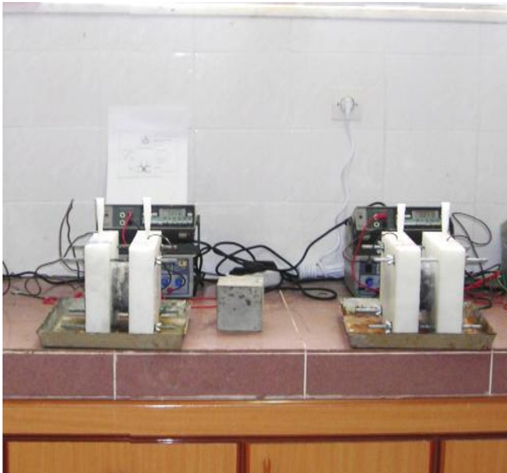
Figure 3.8 Photographic view of the RCPT test set up
