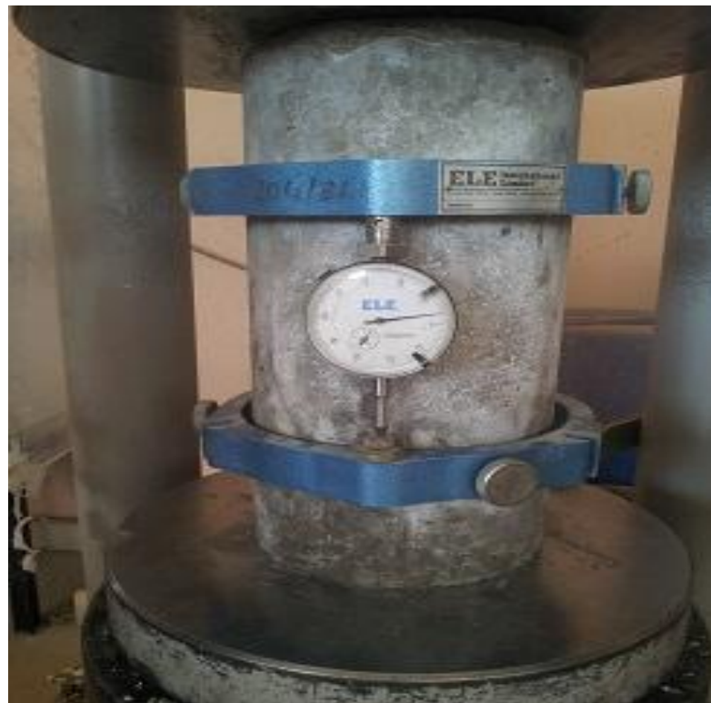
Figure 3.4 Concrete specimen setting for elastic modulus measurement according to dial gage cable.
