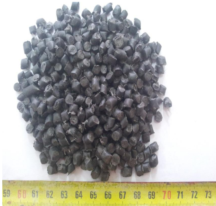
Figure 3.1 Photographic view WRA used in the production of SCRC
