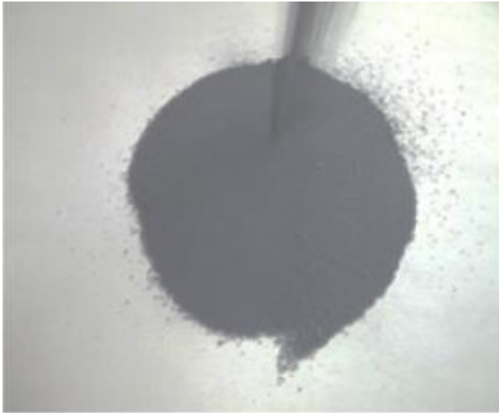
Figure 2.5 Photographic view of silica fume (Yajun and Cahyadi, 2003)
