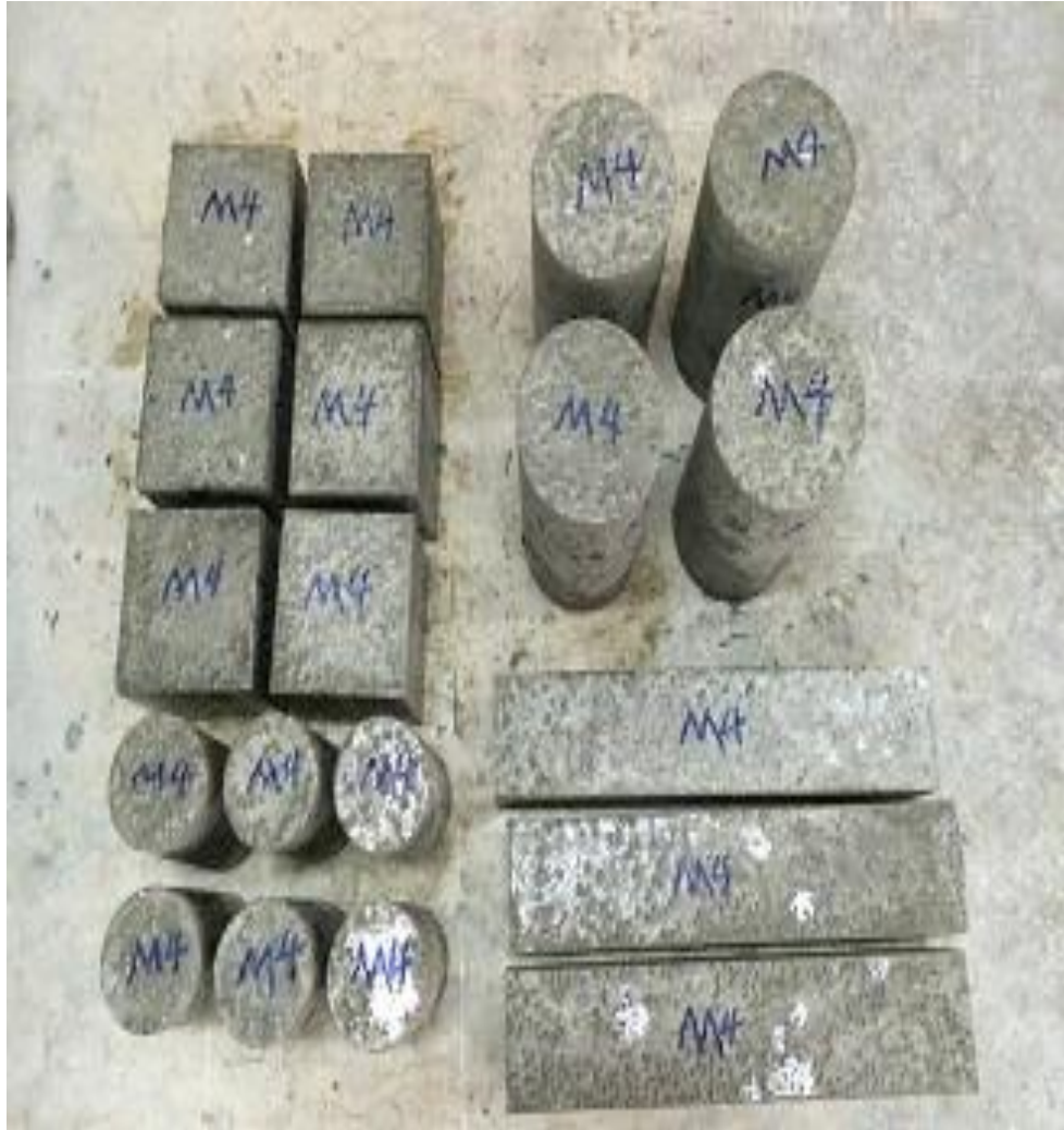
Figure 3.2 Casting of self-compacting rubberized concrete specimens
