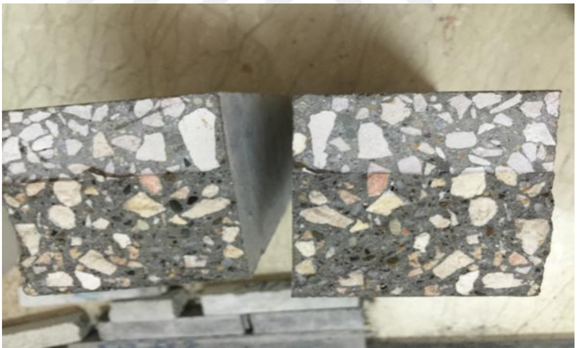
Figure 3.9 The shape of the concrete cube after conducting the fracture energy test.
