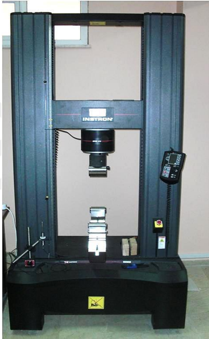
Figure 3.7 Photographic view of testing devices and three-point flexural testing fixture.
