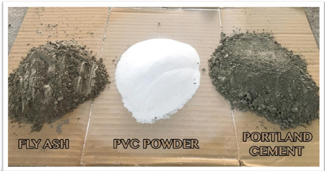
Figure 3.1 Photographic views of FA, PVC powder and PC used in production of SPC
