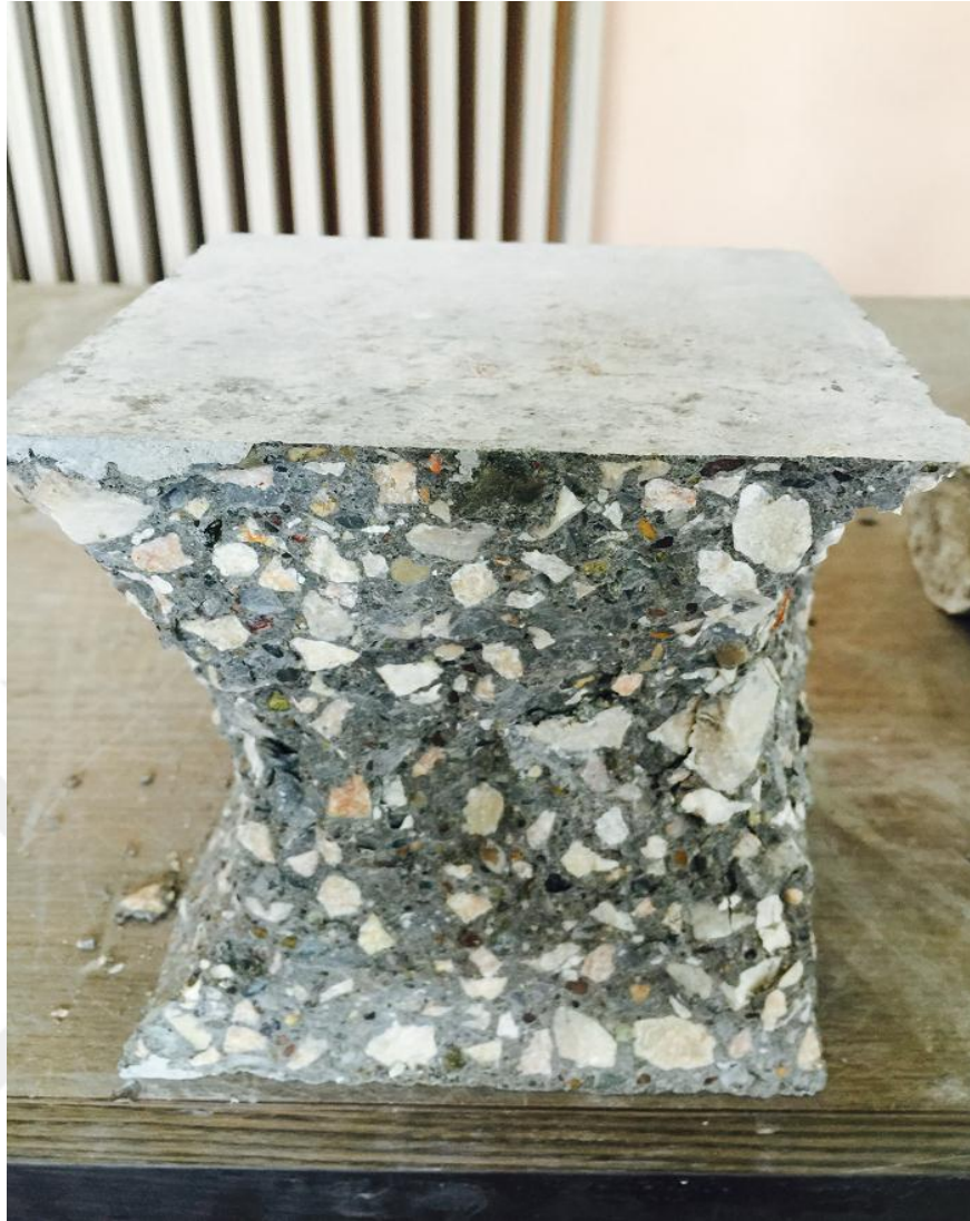
Figure 3.3 The shape of the concrete cube after conducted the compressive strength test.
