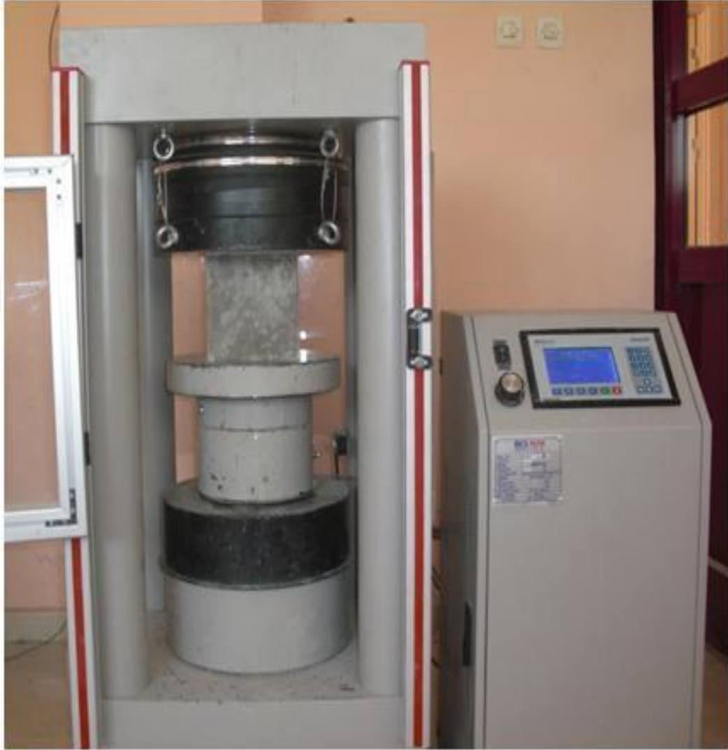
Figure 3.2 When conducting compressive strength test.
