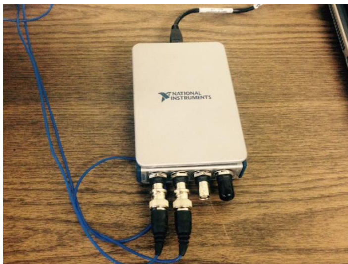
Figure 3.17 Data Acquisition Card (DAQ) Specific Functions of NI 9234 DAQ
