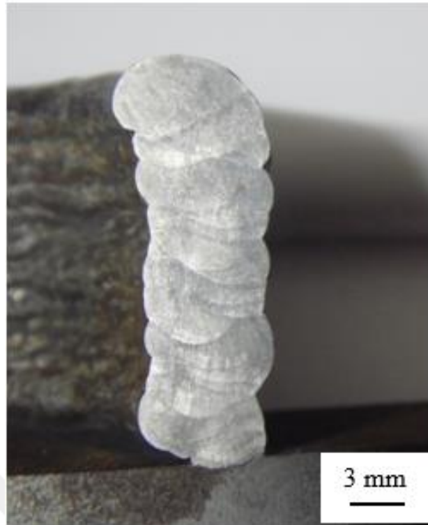
Figure 4.6. Macrograph shows the cross-section of the deposited wall experiment 3 (I=90 A, TS=0.1 m/min, WFS=1.9 m/min)
