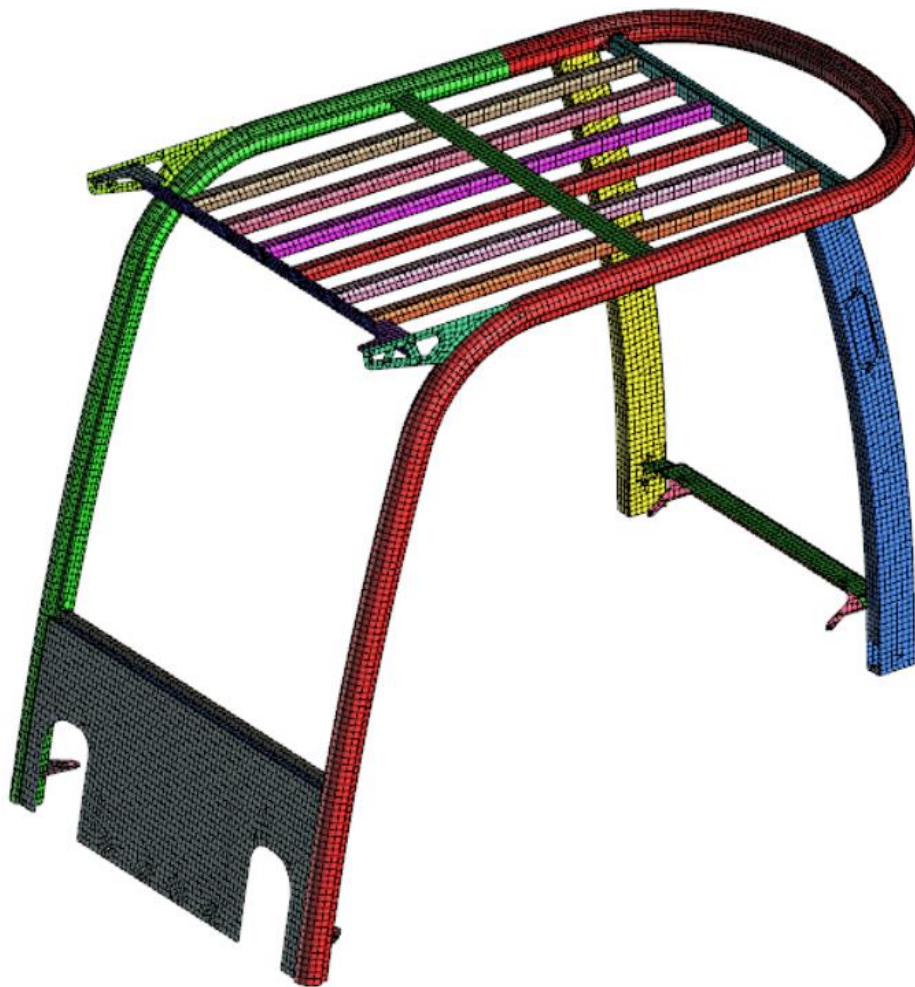
Figure 4.13. Finite element model of head-guard.
