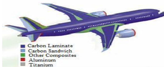
Figure 3.2 : Use of composite materials in different bodies of an aircraft [16]
