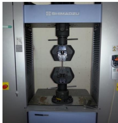
Figure 4.3 : Universal test machine for tensile test
