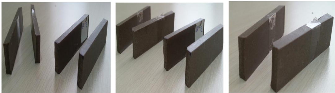
Figure 5.8 : Typical Failed Specimen for Three Point Bending Test
