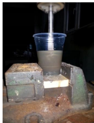
Figure 4.2 : Reaction of polyester and hardener
