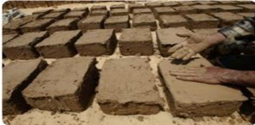
Figure 3.3 : Production of adobe material [15]
