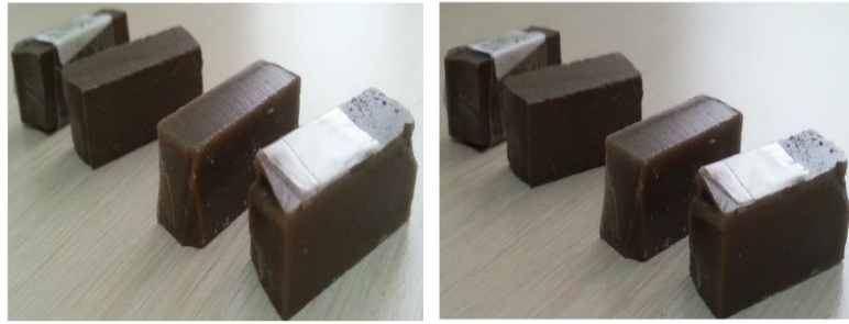
Figure 5.11 : Typical Failed Specimen for Impact Test
