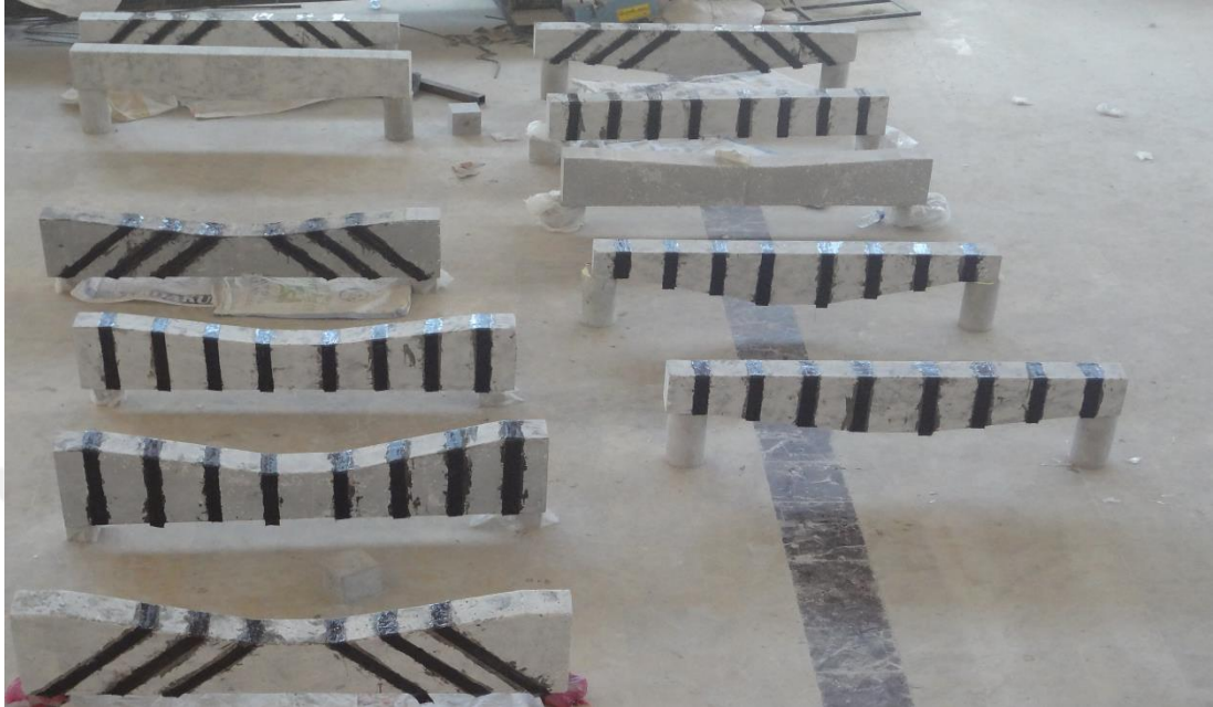
Figure 3.16 Curing of all beams after strengthening.
