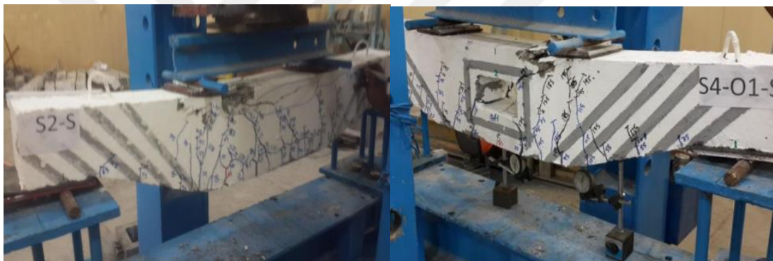
Figure 2.5 Types of failure after strengthening(Dawood & Nabbat 2015). where is this reference in text.
