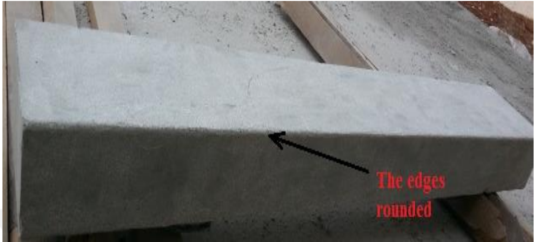
Figure 3.10 Rounded bottom edge in order to reduce the stress concentrations on the CFRP strip
