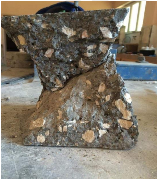
Figure 4.8 Compressive strength type failures at 90 days
