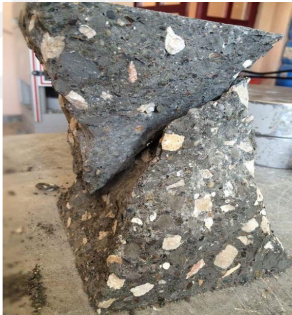
Figure 4.8 Compressive strength type failures at 90 days
