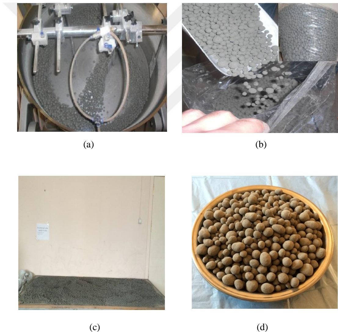
Figure 3.3 Views of a) pellets agglomerate after approximately 20 minutes b) Self-curing process c) Sieving process d) Fly ash lightweight aggregate
