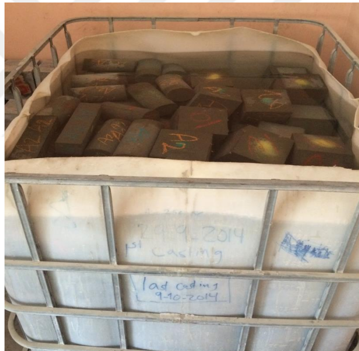
Figure 3.8 Specimens in water curing
