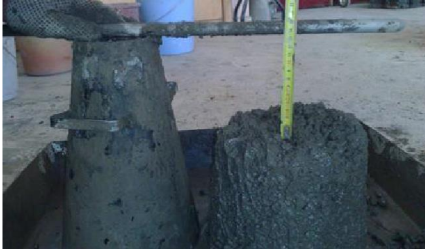
Figure 3.7 Slump test for LWACs mixtures
