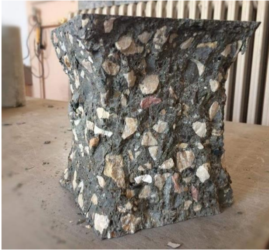
Figure 4.7 Compressive strength type failures at 28 days
