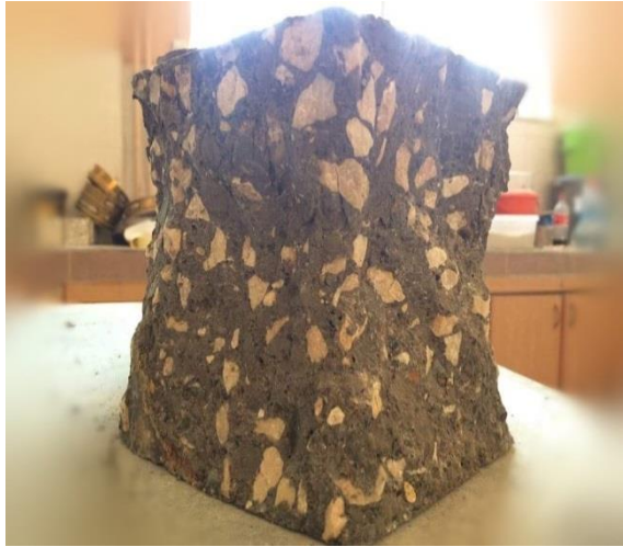
Figure 4.7 Compressive strength type failures at 28 days
