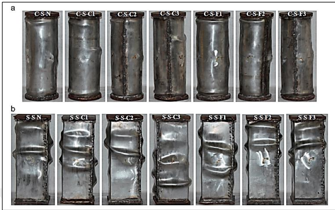
Figure 2.24 The failure patterns of CFST specimen columns (a) Circular section. (b) Square section. (Yang and Ma, 2013)
