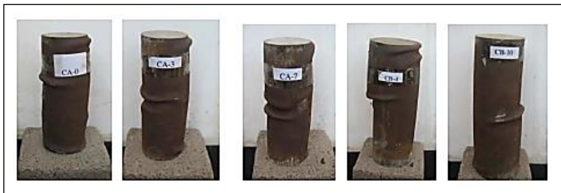
Figure 0.23 The failure patterns of CFST specimen columns (Chen et al., 2010)
