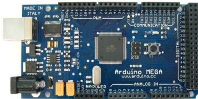
Figure 2.11: Arduino Mega 1280 / 2560 board [25]
