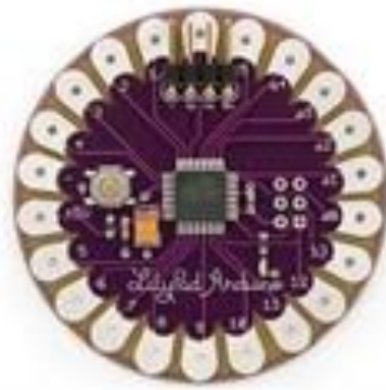
Figure 2.5: Arduino LilyPad board [25]
