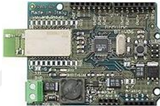
Figure 2.10: Arduino Bluetooth board [25]
