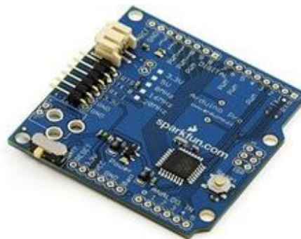
Figure 2.7: Arduino Pro 3.3V / Pro 5V board [25]
