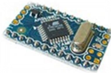
Figure 2.1: Arduino Mini/Mini Lite board [25]
