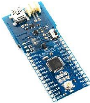
Figure 2.4: Arduino Fio board [25]
