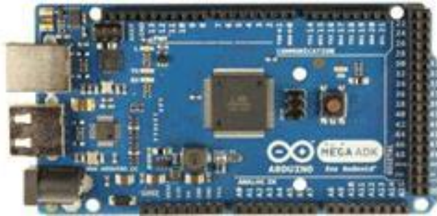
Figure 2.12: Arduino Mega ADK 1280 / 2560 board [25]
