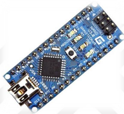
Figure 2.3: Arduino Nano / Nano Lite board [25]
