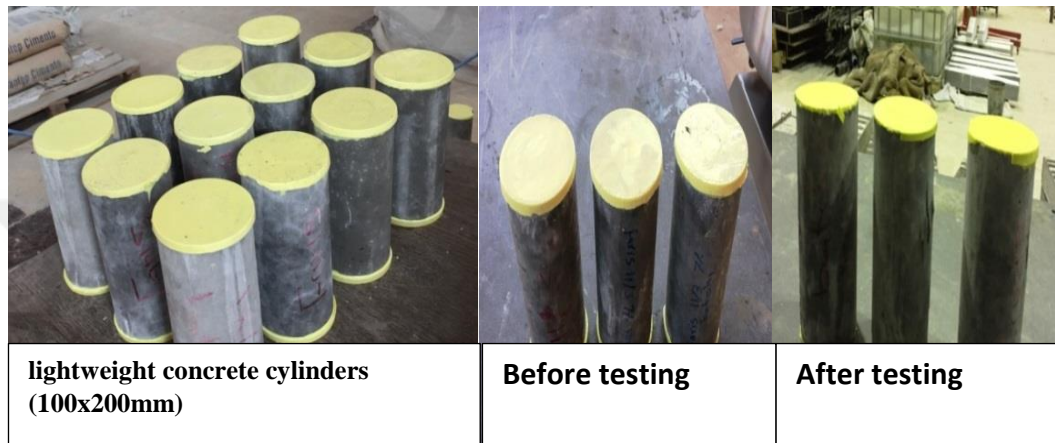
Figure 4.3 Casting and testing the Cylinders
