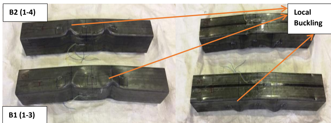
Figure 4.12 Local buckling for hollow section beams
