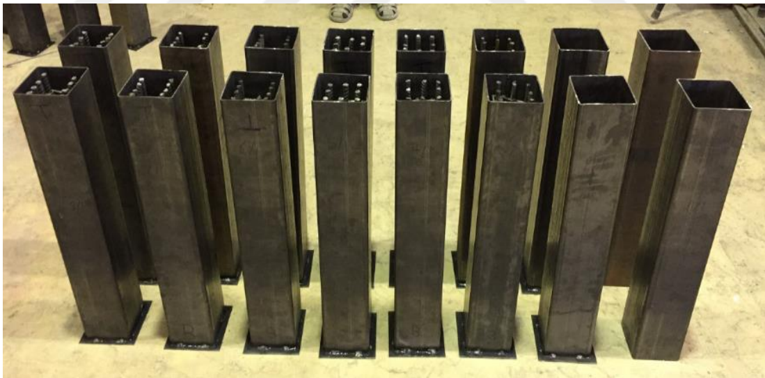
Figure 1.1 Sixteen beam specimens of square section for this study
