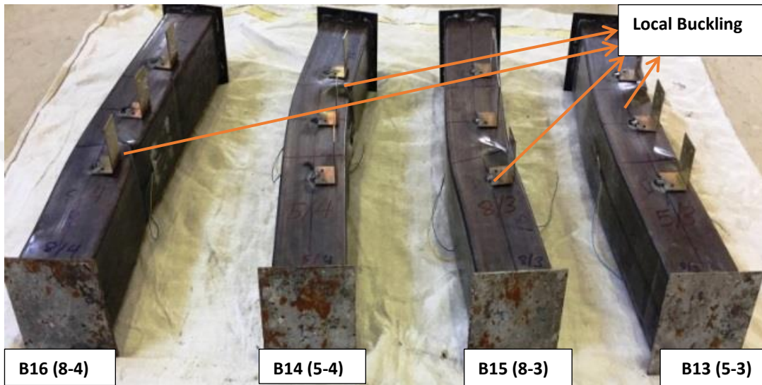
Figure 4.20 Local backing for RCFST ( \rho= 7\% ) beams
