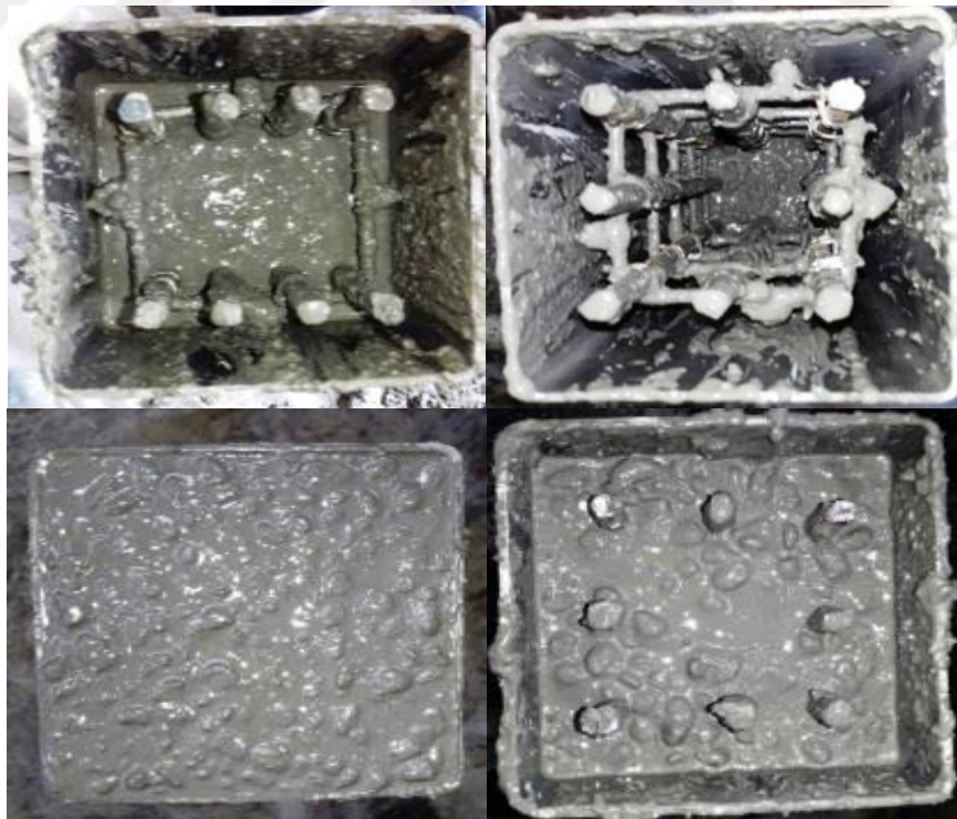
Figure 4.9 Casting the specimens
