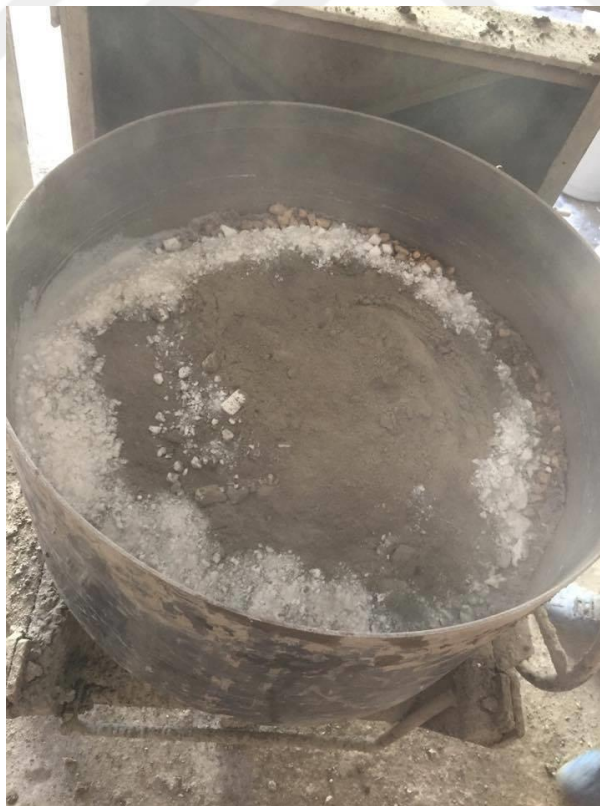
Figure 3.5 Adding Cementitious material to fine and coarse aggregate mix
