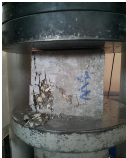
Figure 4.2 Photographic view of compressive strength of concrete test at 28 days
