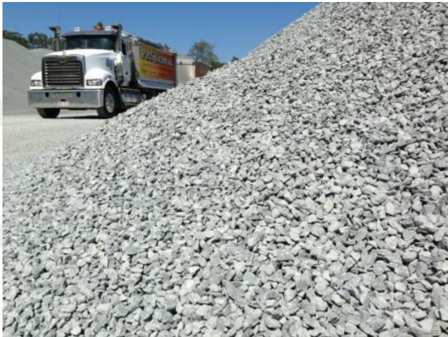
Figure 2.4 Photographic view of Natural Coarse aggregate
