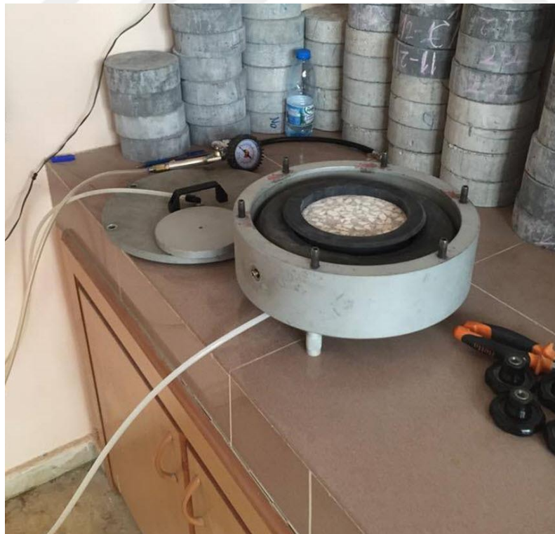
Figure 3.16 Photographic view of gas permeability specimen in the cell
