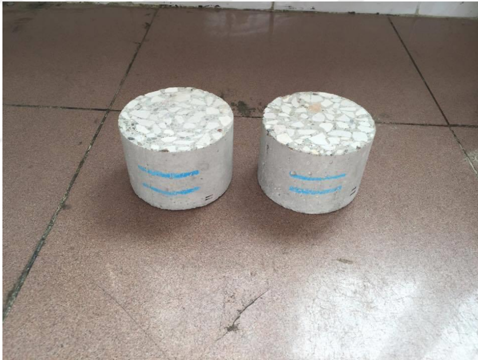
Figure 3.11 Photographic view of water sorptivity specimens after rying
