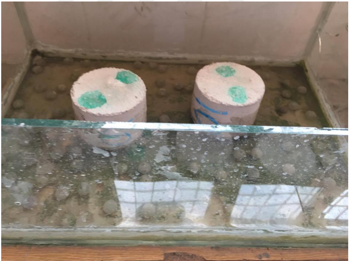
Figure 4.4 Photographic view of water Sorptivity of concrete at 28 days
