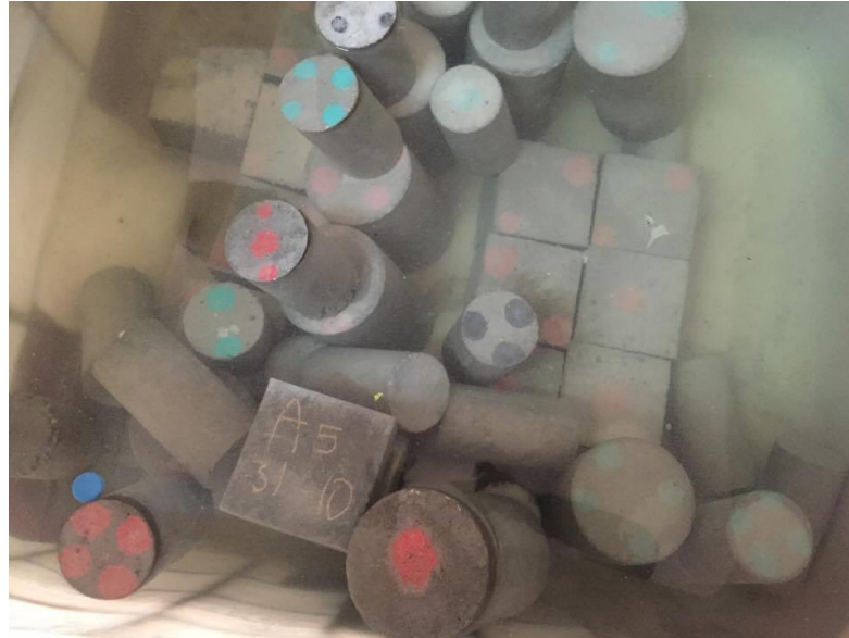
Figure 3.7 Photographic view of specimens at curing time
