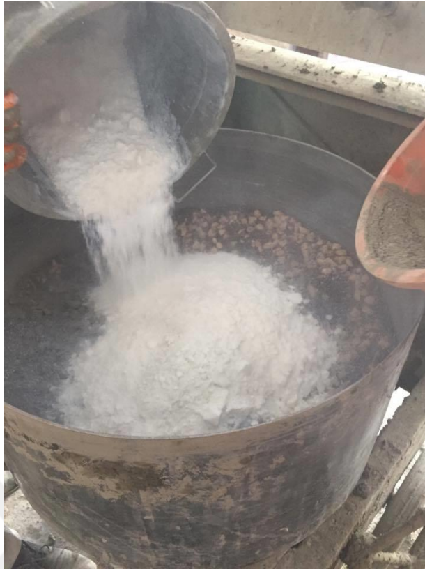
Figure 3.5 Adding Cementitious material to fine and coarse aggregate mix
