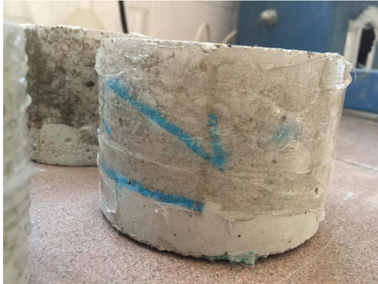
Figure 3.12 Photographic view of water Sorptivity specimens after coating by silicone
