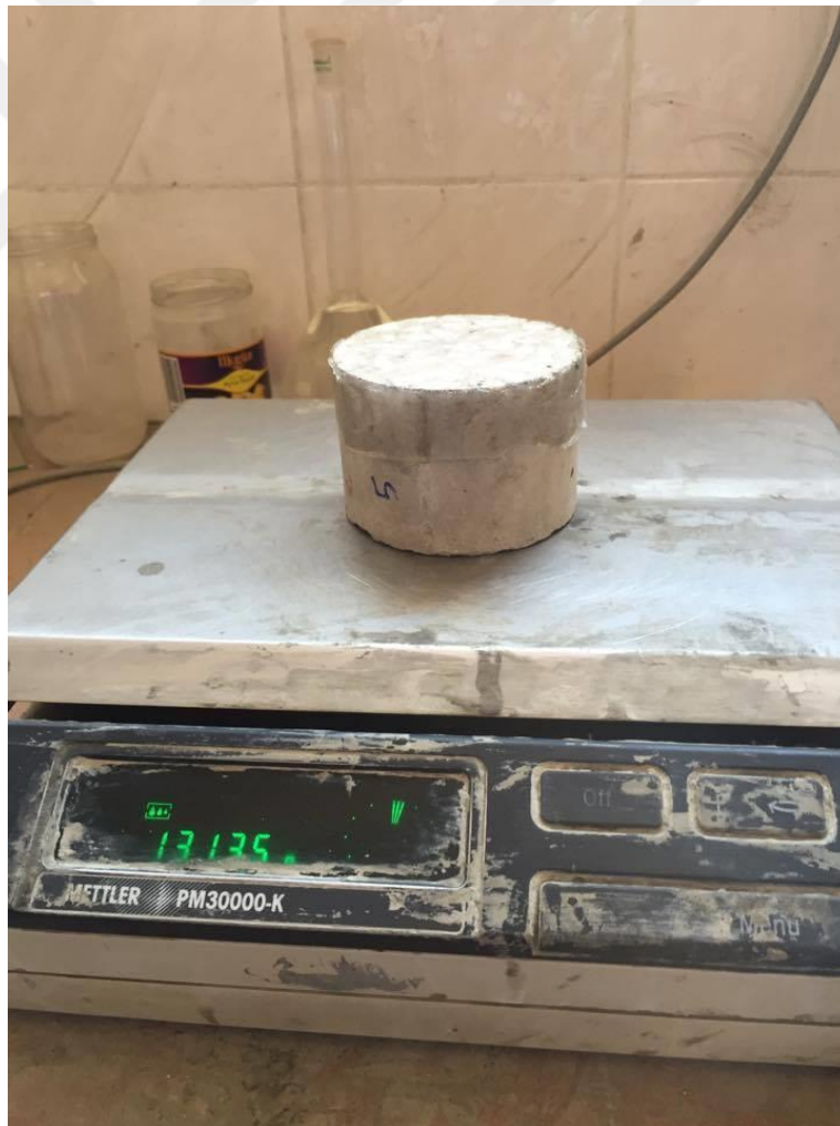
Figure 3.12 Photographic view of water Sorptivity specimens after coating by silicone
