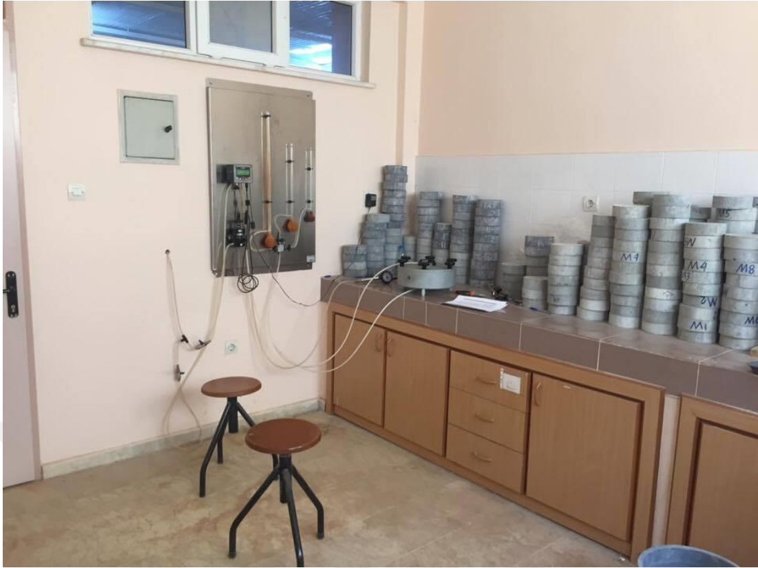
Figure 3.19 Photographic view of gas permeability test
