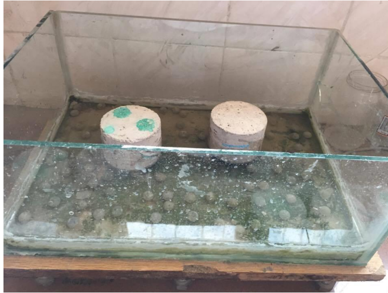
Figure 3.14 Photographic view of water Sorptivity specimens at testing time
