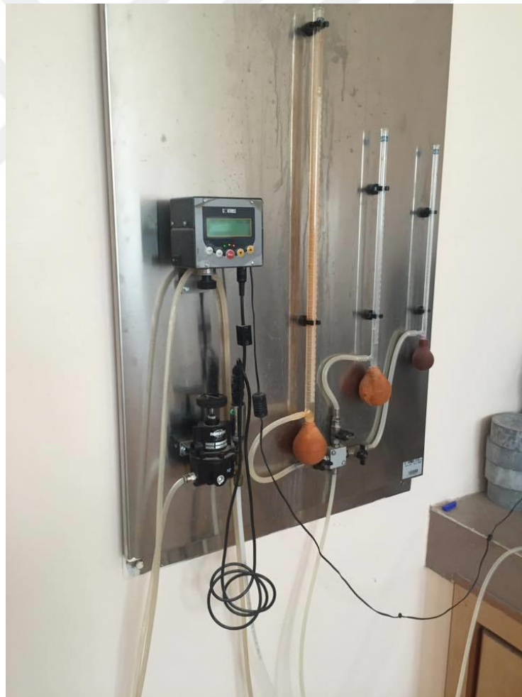
Figure 3.18 Photographic view of gas permeability at testing time
