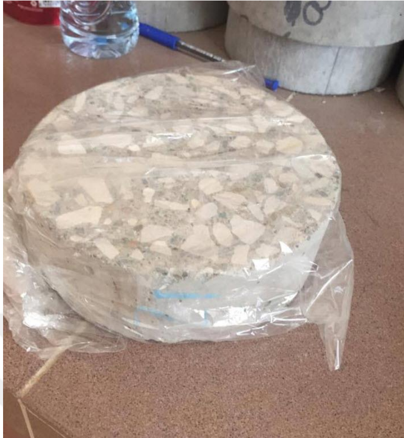
Figure 3.15 Photographic view of gas permeability specimen after drying
