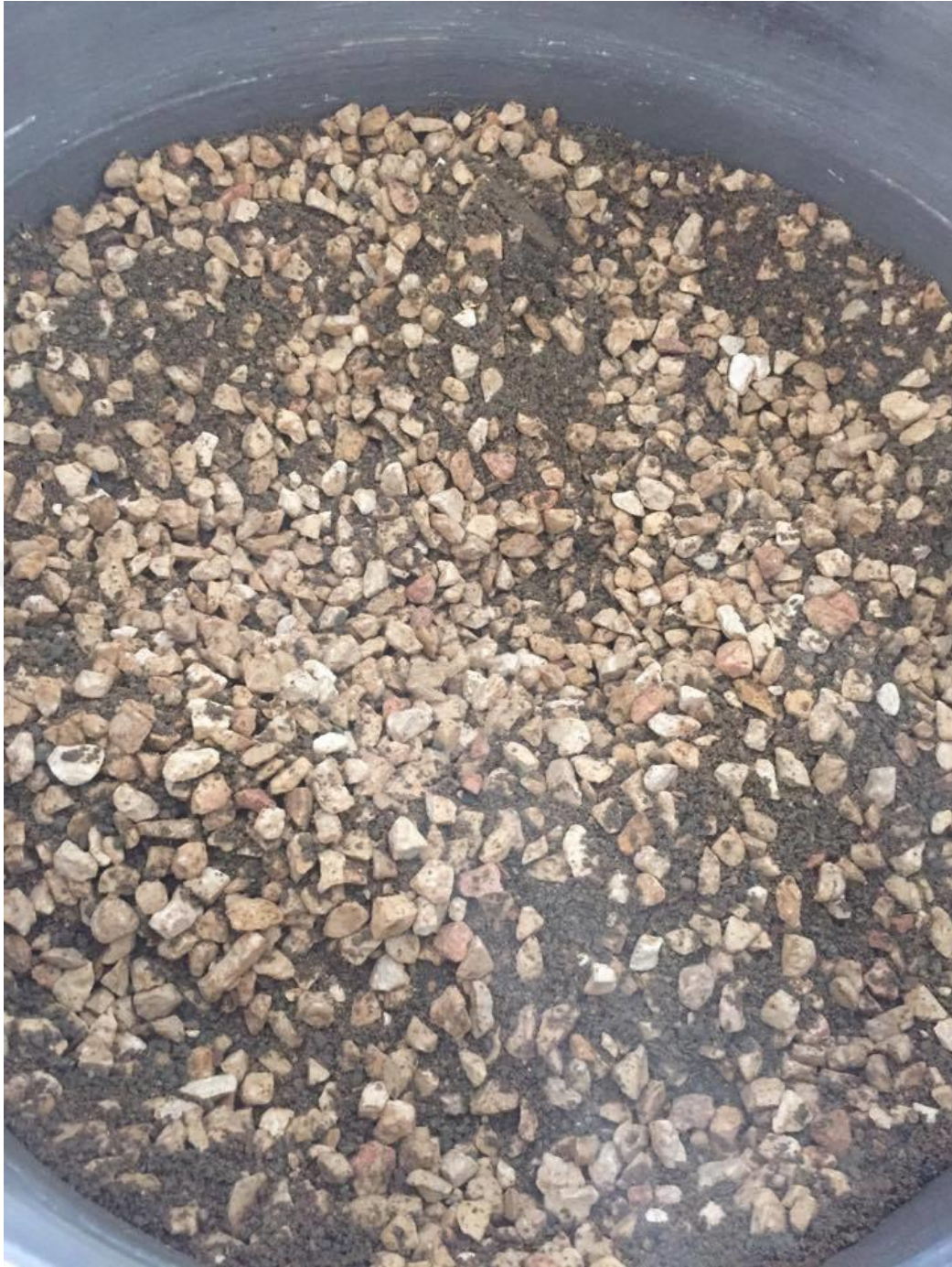
Figure 3.4 Mixing of fine and coarse aggregate
