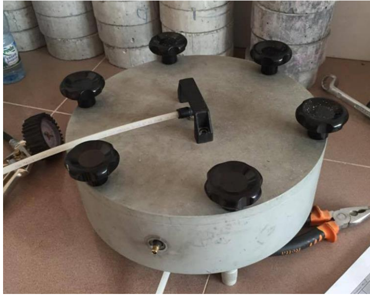
Figure 3.17 Photographic view of gas permeability specimen at testing time
