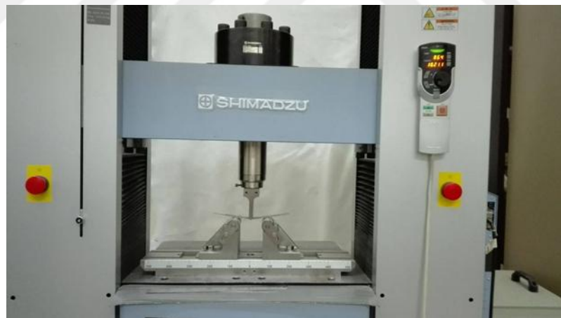
Figure 3.10 Test set-up Shimadzu AG-X series testing machine (flexural test)
