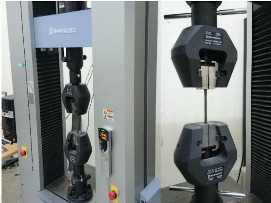
Figure 3. 8 Test set-up Shimadzu AG-X series testing machine (tensile test)
