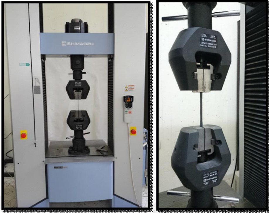
Figure 3.9 (a) tensile test set-up, (b) specimen under test.
