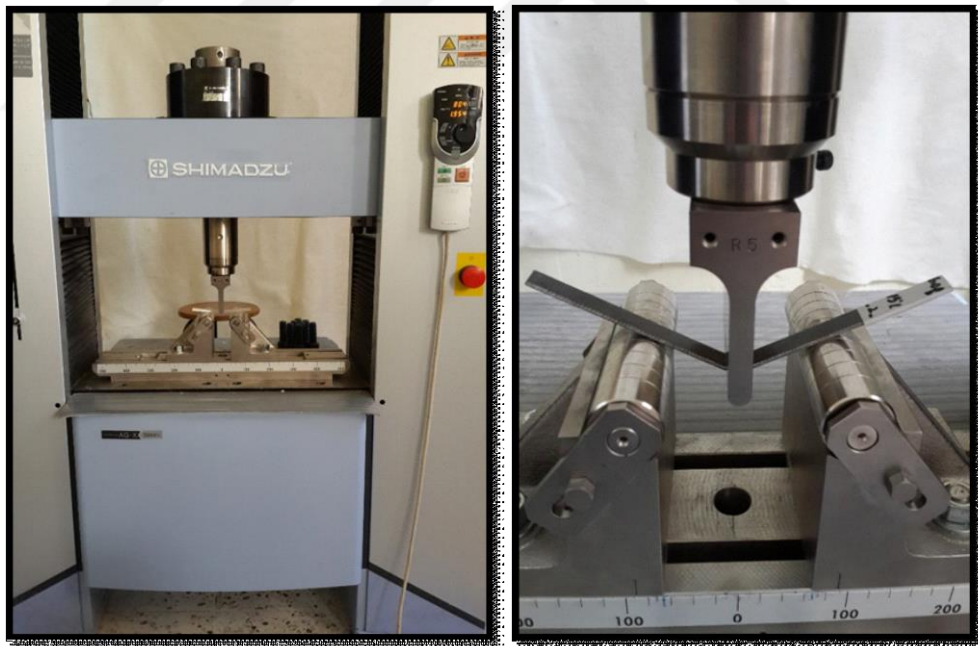
Figure 3.10 (a) flexural test method, (b) specimen under test.
