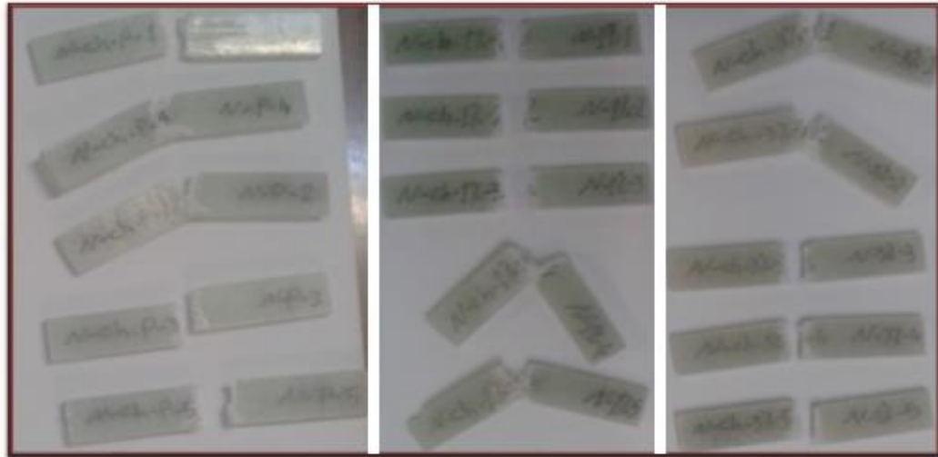
Figure 4.4 Sample of edgewise specimen after test ( G_{12} ).
