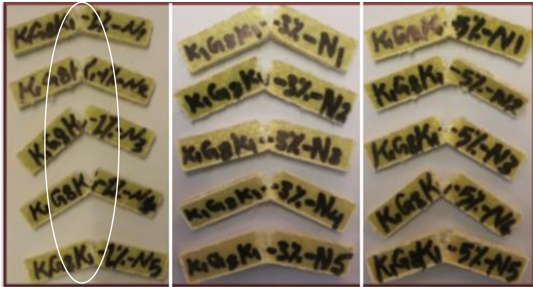
Figure 4.20 Sample of the edgewise specimen of [K_1G_4]_s after test.
