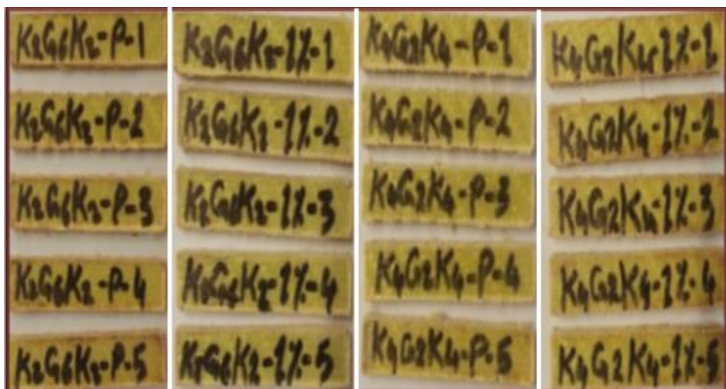
Figure 4.15 Sample of the flatwise specimen of hybrid with 0 wt.% and 1wt.% nanoclay before test.
