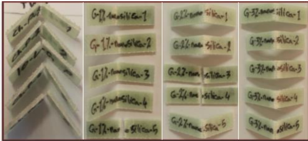
Figure 4.32 Sample of the flatwise specimen of glass with nanosilica after test.
