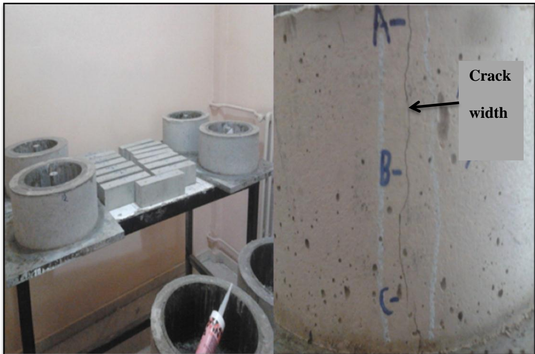
Figure 3.6 Photographic view of restrained shrinkage samples
