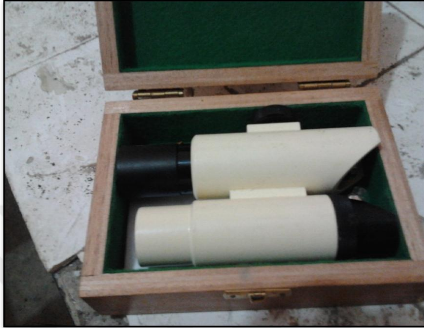
Figure 3.5 Photographic view of crack width measurement apparatus
