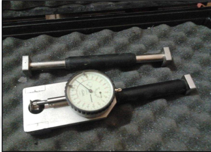
Figure 3.3 Photographic view of dial gage extensometer apparatus
