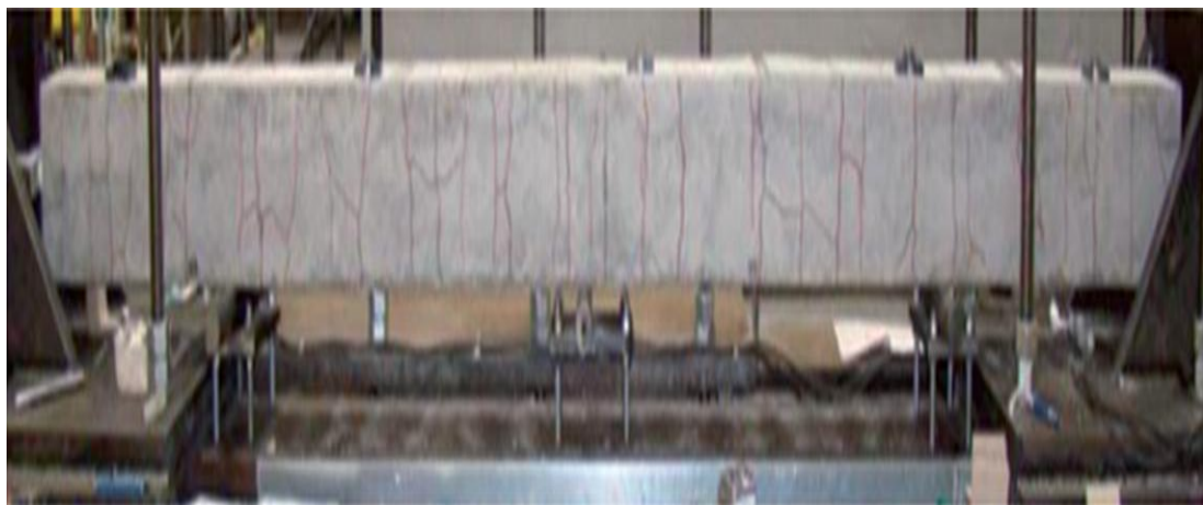
Figure 1.4 Tie with one reinforcement bar at crack saturation stage (French national research program, 2014)
