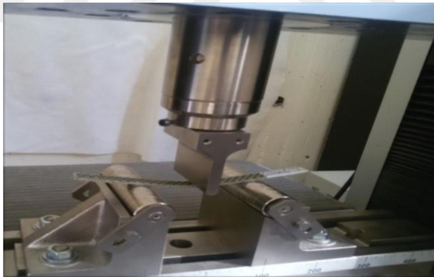
Figure 3.13 Flexural test set-up Shimadzu AG-X arrangement testing machine.
