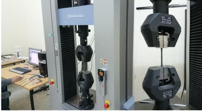
Figure 3.11 Tensile test set-up Shimadzu AG-X arrangement testing machine.
