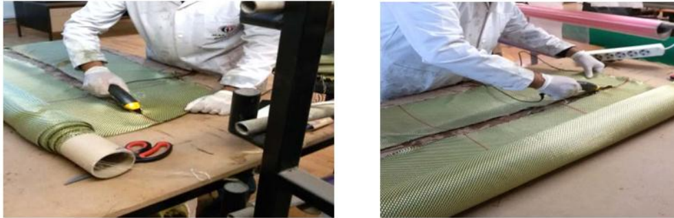
Figure 3.4 Cutting fibers by EC, Carbon/Kevlar fiber.
