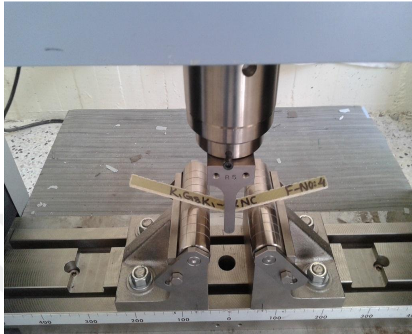
Figure 3.22 Test set-up Shimadzu AG-X series testing machine (flexural test)
