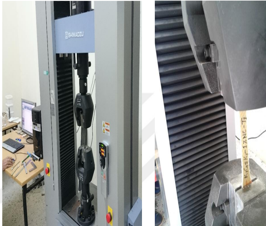
Figure 3.19 Test set-up Shimadzu AG-X series testing machine (tensile test)
