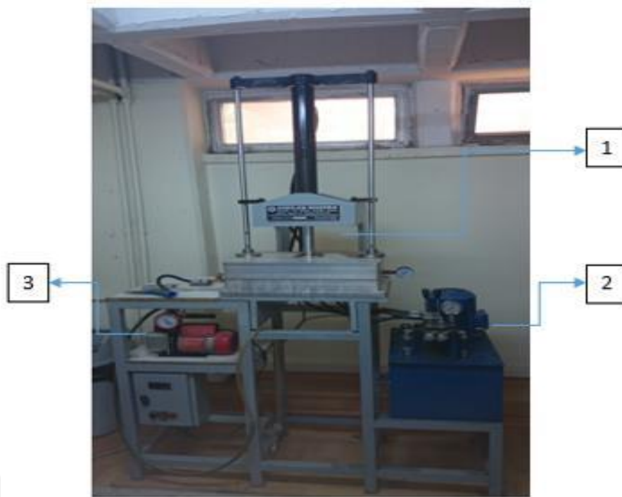
Figure 3.12 Hot press. (1) Combination of heat pressure and vacuum (2) Hydraulic unit (3) Vacuum pump
