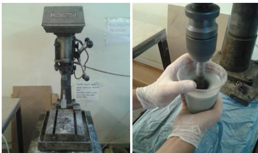
Figure 3.9 Mixing process of epoxy resin and nano-clay
