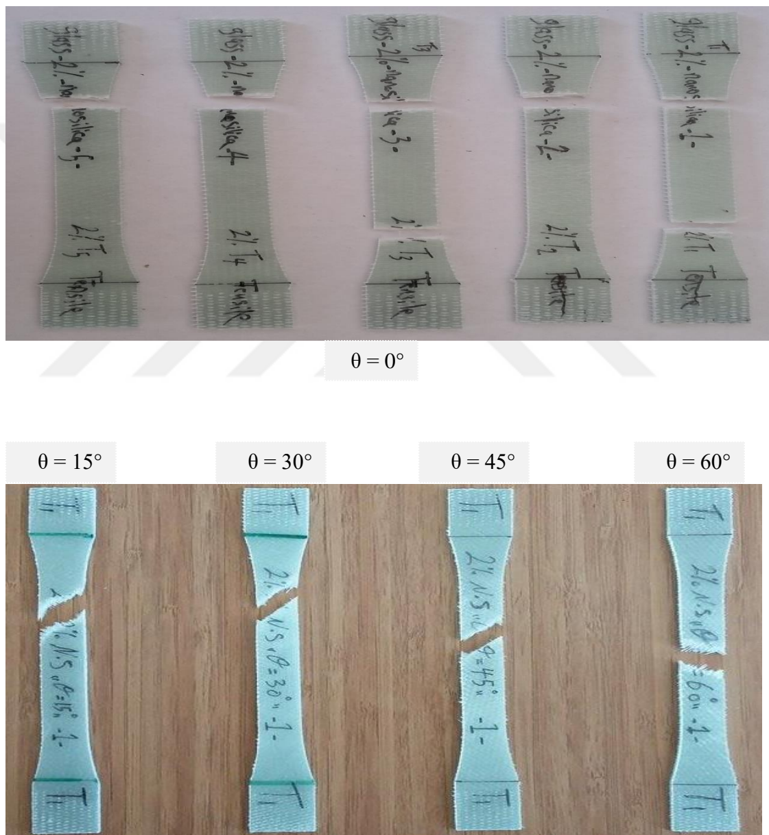
Figure 4.15 Failure specimens at 2wt% nanosilica content with different fiber orientation angles after tensile test
