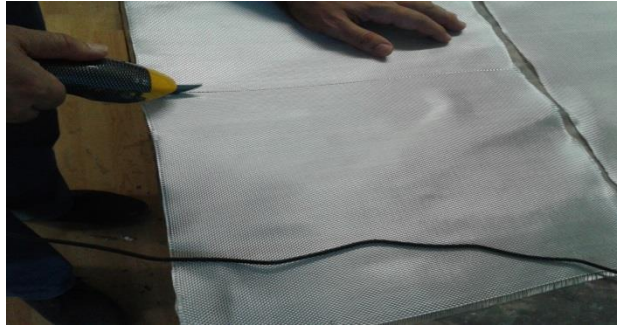
Figure 3.4 Cutting fibers by EC, Glass fiber
