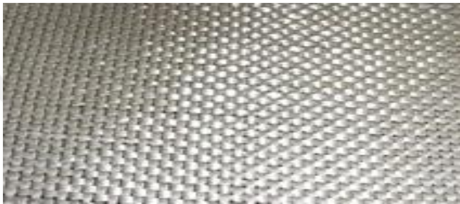
Figure 3.2 Woven E-glass fiber utilized in this study
