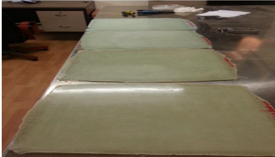
Figure 3.7 Examples of producing nanocomposite laminate
