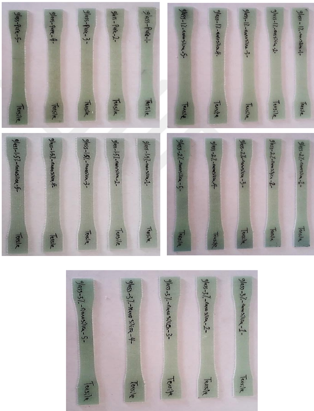
Figure 3.9 GFRE-NS composite samples for tensile test
