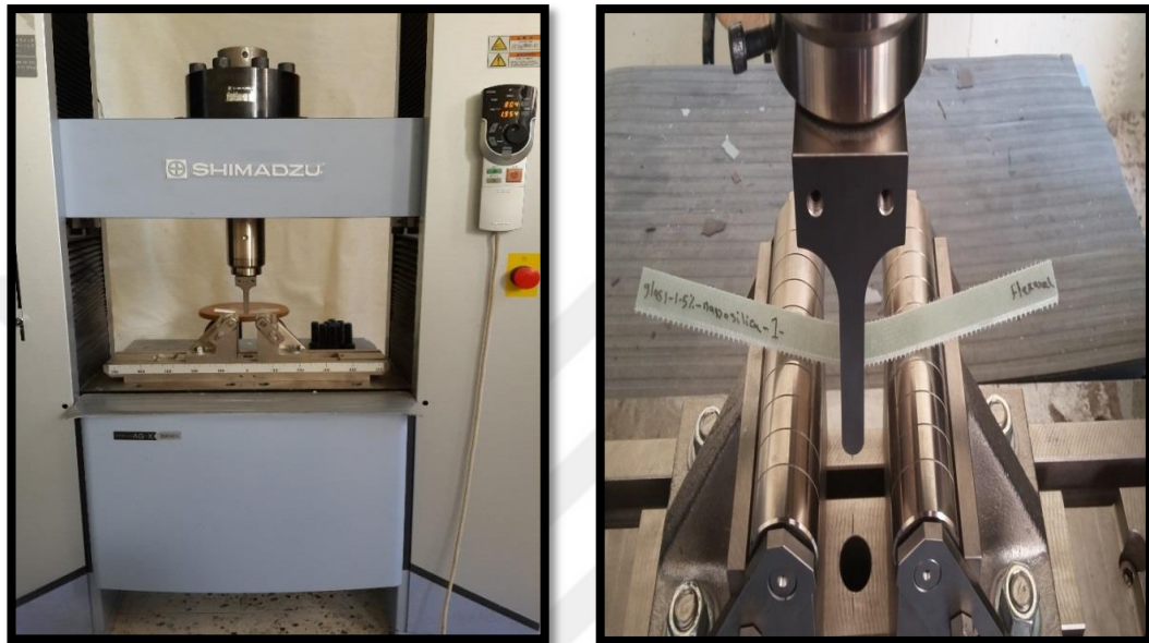
Figure 3.15 The flexural test device (Shimadzu AG-X testing)
