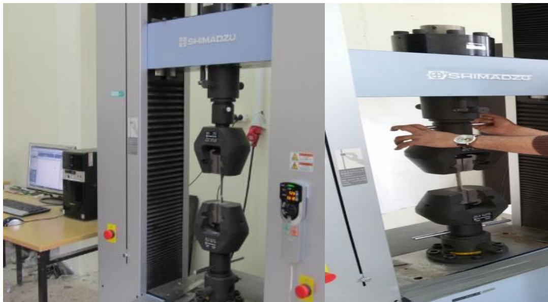
Figure 3.12 Tensile test set-up Shimadzu AG-X arrangement testing machine
