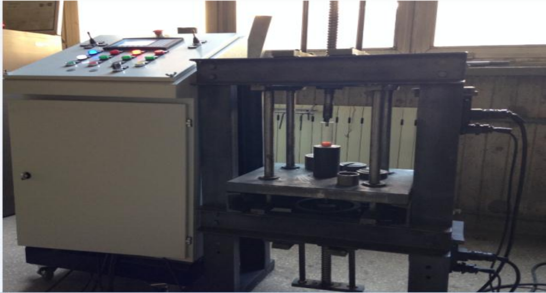
Figure 4.8 Photograph of the servo-press used in forging experiment
