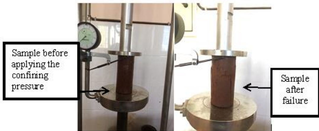
Figure 3.16 The unconfined compressive strength sample before and after applying the load.
