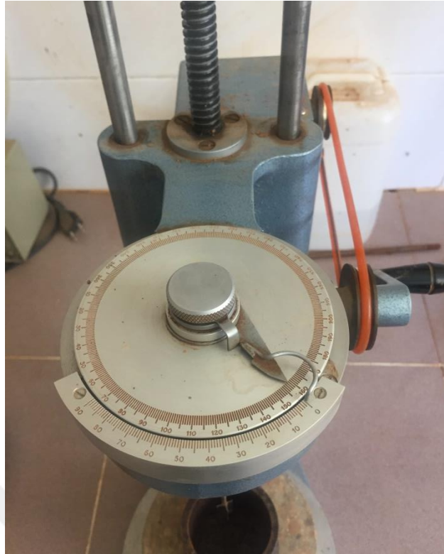
Figure 3.21 Calibrated scale of vane shear device used during the experimental study
