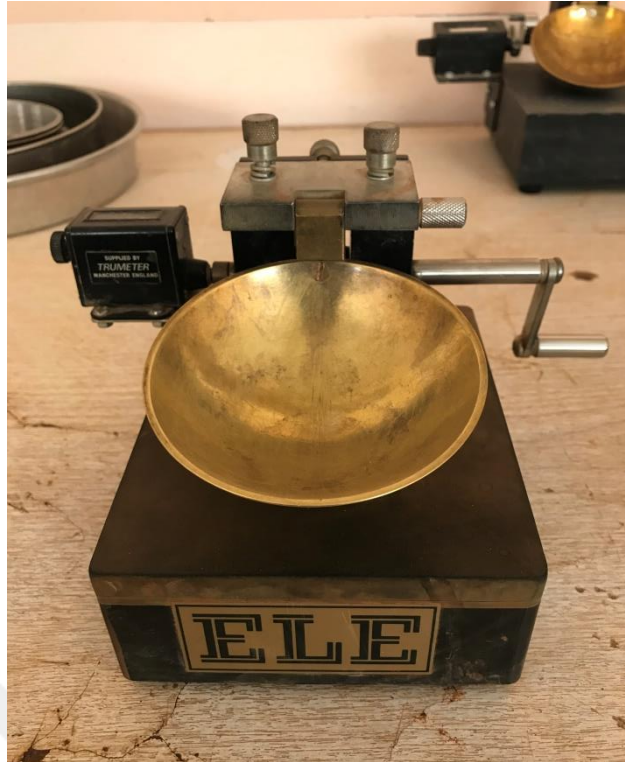
Figure 3.13 Casagrande device used during the experimental study.
