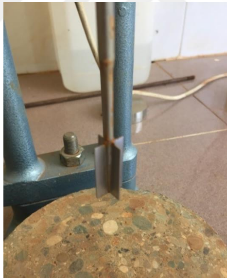
Figure 3.20 The blades of laboratory vane shear device used during the experimental study
