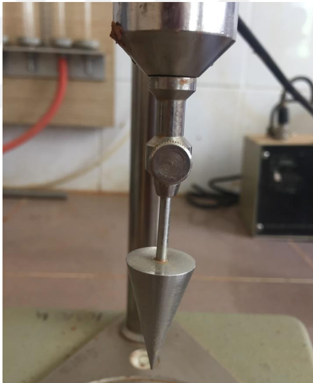
Figure 3.18 The stainless steel penetration cone
