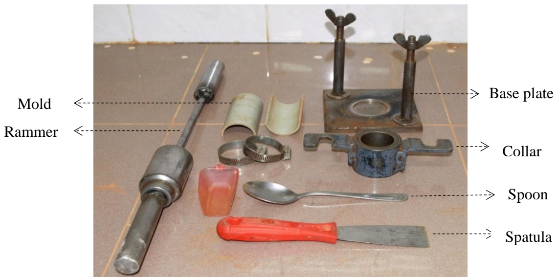
Figure 3.6 The plastic split mold and the compaction hammer for the modified compaction test
