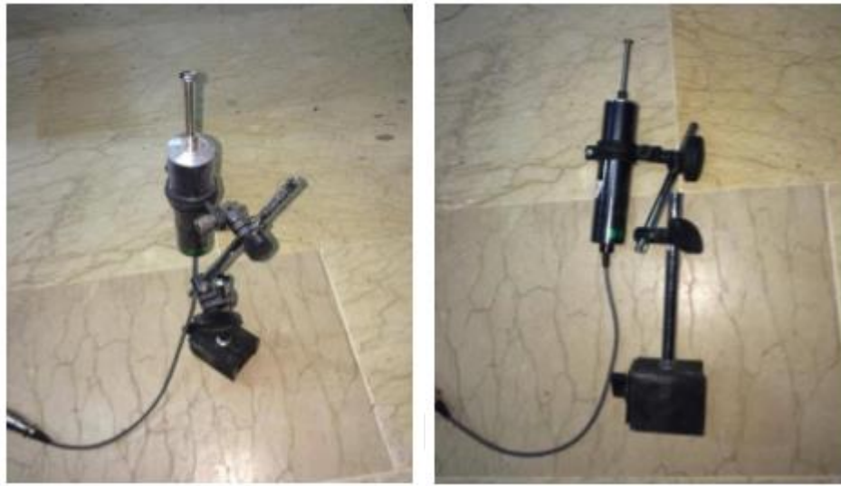
Figure 4.2 LVDT (Linear variable differential transformer)
