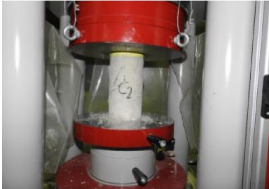
Figure 3.8 Cylinder compressive test
