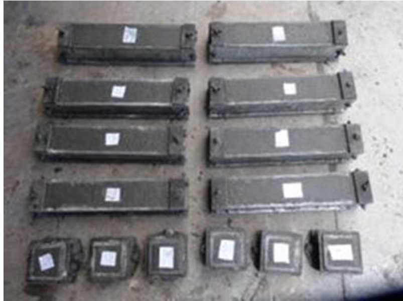
Figure 3.11 Casting the mixture in the cube & prism mould
