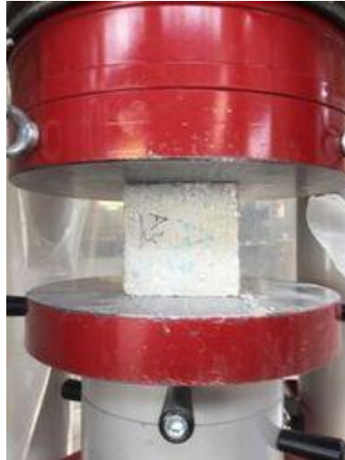
Figure 3.19 Sample of compressive strength
