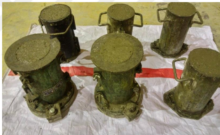
Figure 3.12 Casting mixture in the cylinder moulds
