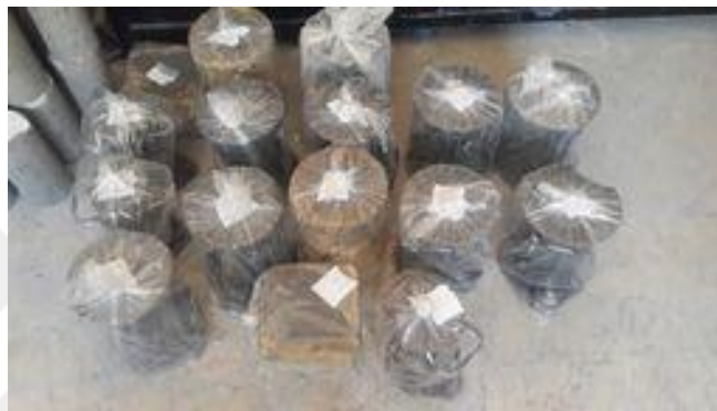
Figure 3.13 a,b Covering the moulds with plastic bags
