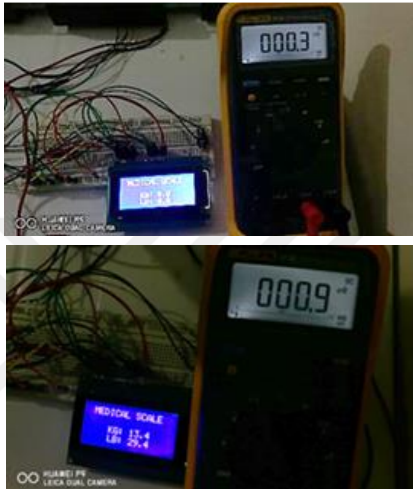
Figure 4.21 Load cell bridge output voltage test
