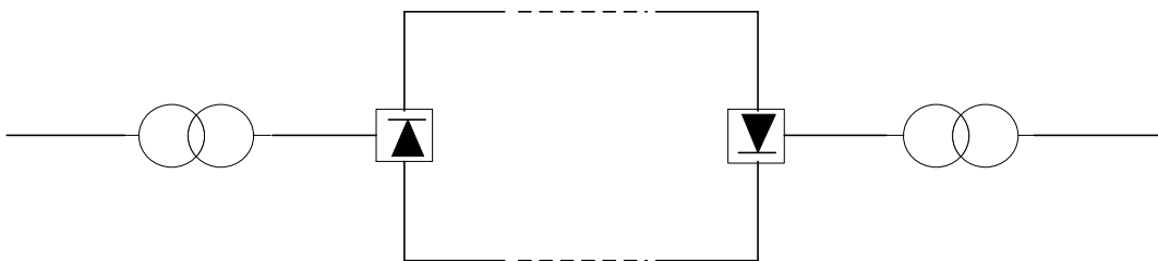
Figure 2.7 Back-to-back configuration of HVDC system
