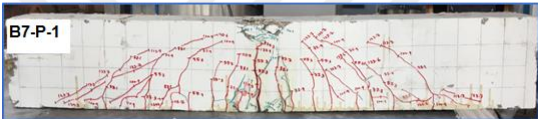
Figure 4.7 Flexural Failure for Beam (B7-P-1)
