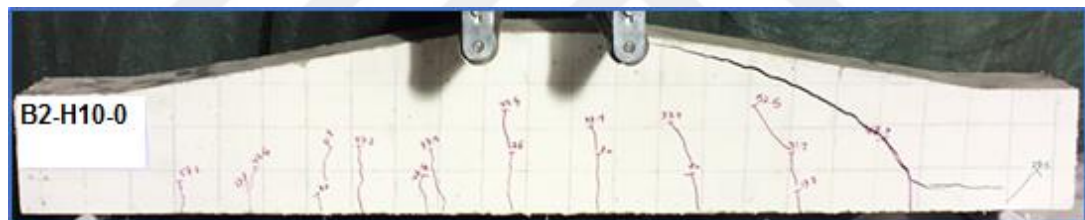
Figure 4.2 Shear Failure for Beam ( B2-H10-0)
