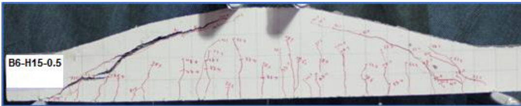
Figure 4.6 Shear Failure for Beam (B6-H15-0.5)
