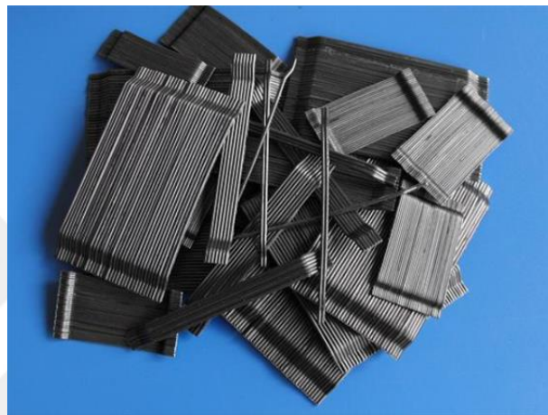
Figure 3.2 Steel Fiber Hook-end
