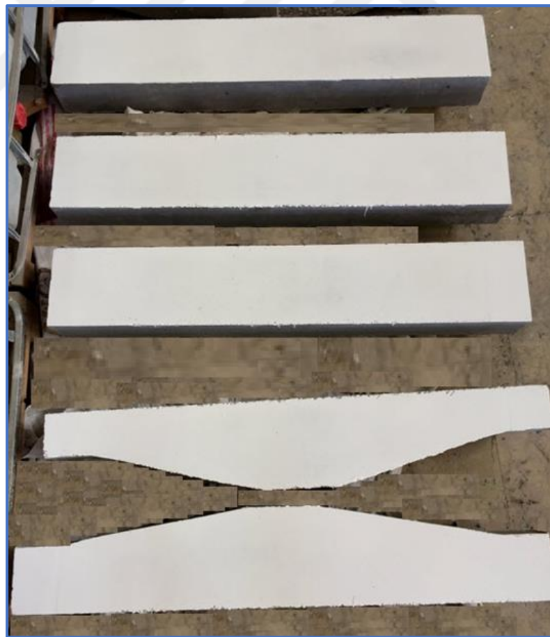
Figure 3.12 painting and Preparing Beams before Testing.
