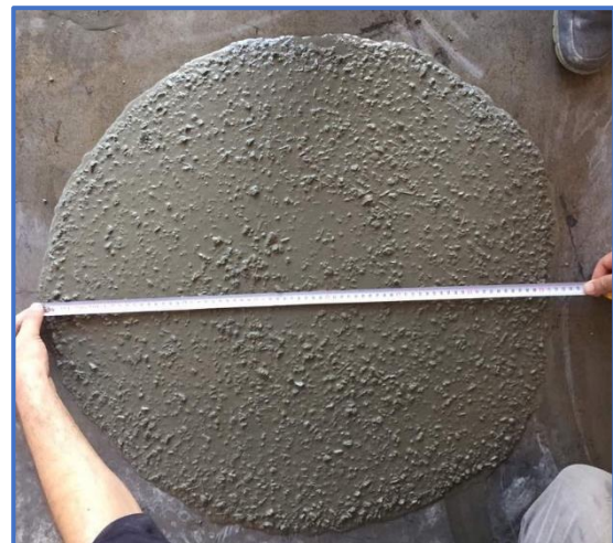
b. The Test of the Slump Flow
