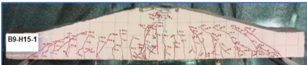
Figure 4.9 Flexural Failure for Beam (B9-H15-1)
