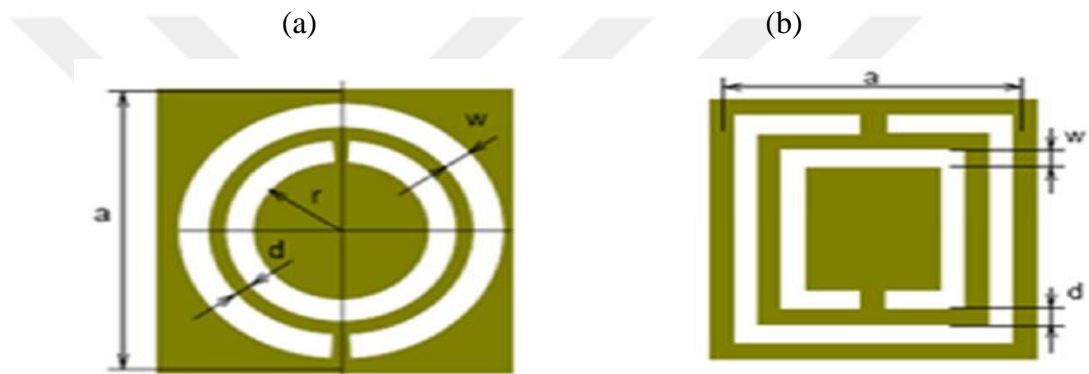
Figure 1.3 Complementary SRR structures: a) circular, b) rectangular [22]
