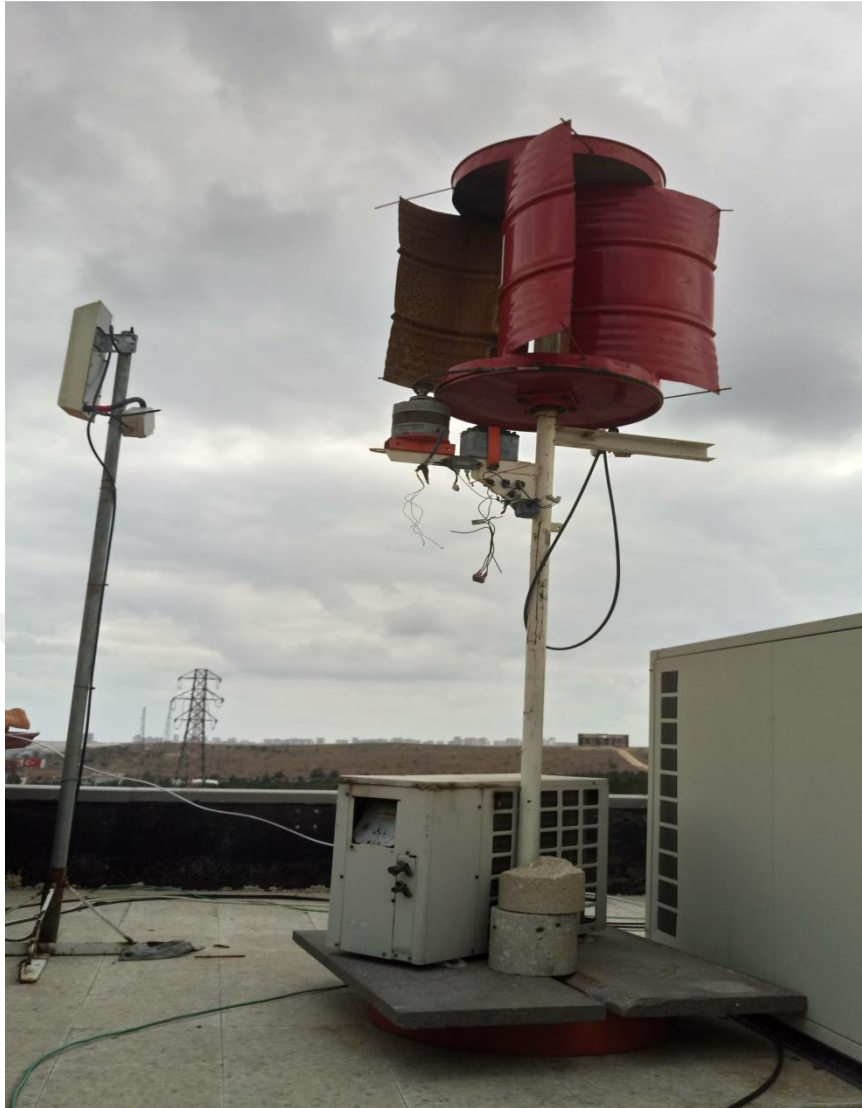
Figure 3.2 Model 2 Savonius with four blades
