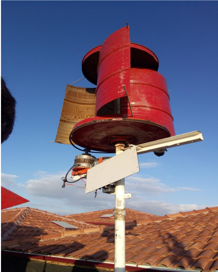
Figure 3.1 Model 1 Savonius with three blades
