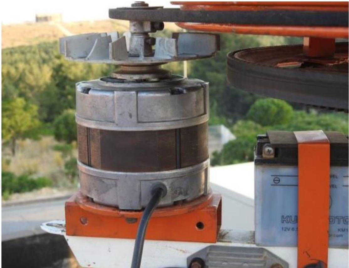
Figure 3.5 The generator placed on the shaft
