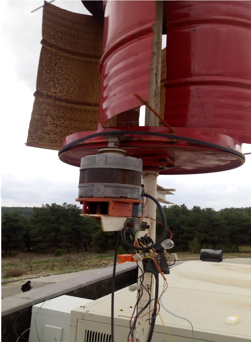
Figure 3.3 The belt and the pulleys in the rotor.
