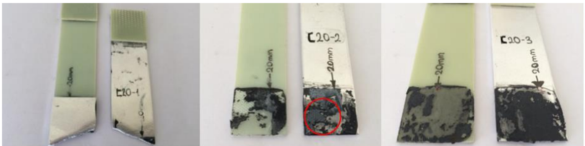
Figure 4.9 C20 Samples after tensile tests
