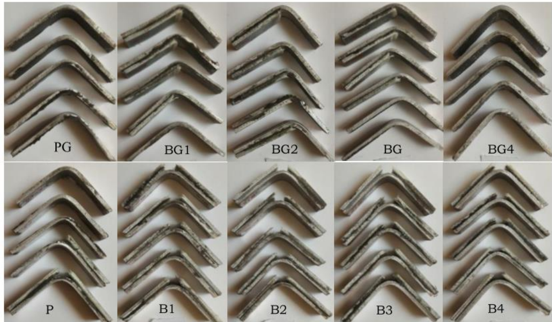
Figure 4.32 View of samples after Charpy impact test of nano-clay doped samples
