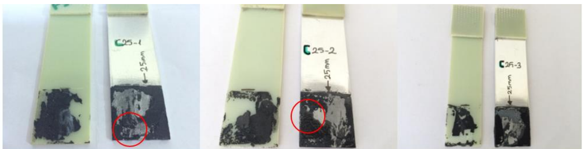
Figure 4.10 C25 Samples after tensile tests
