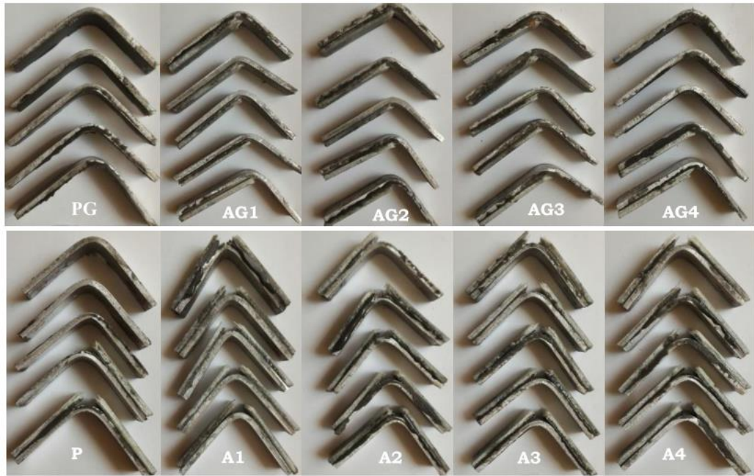
Figure 4.26 Damages' views after Charpy impact test for nano-silica doped samples
