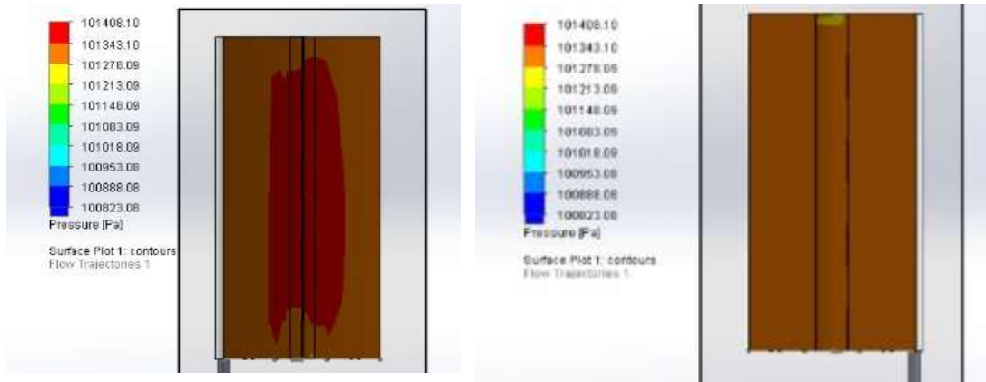
a. Pressure on the front face of the blade b. Pressure on the back face of the blade
