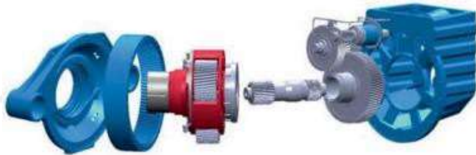
Figure 3.14 Gearbox connecting low-speed shaft to high-speed shaft[ 14]
