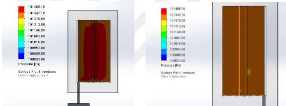
a. Pressure on the front face of the blade b. Pressure on the back face of the blade
