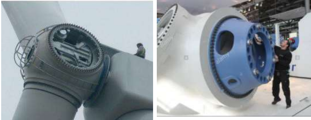
Figure 3.5. Hub in the wind turbine [23]
