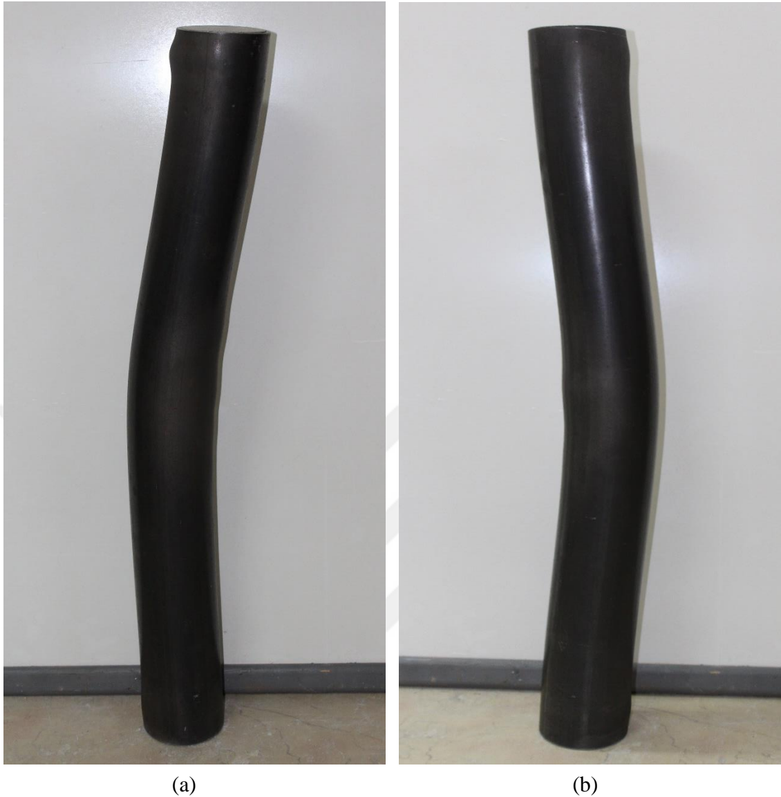
Figure 5.6 Failure modes of 916.5 mm columns (a) F-8-86.53 (b) W-8-92.22.
