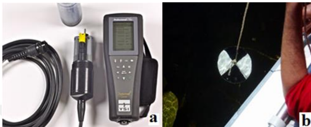
Figure 6.4 Environmental variables sampling a) YSI professional plus, b) Secchi disk
