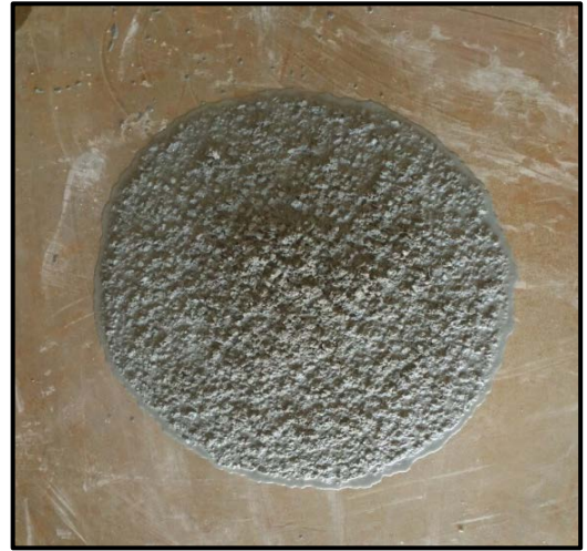
b) Slump flow for 1% SF
