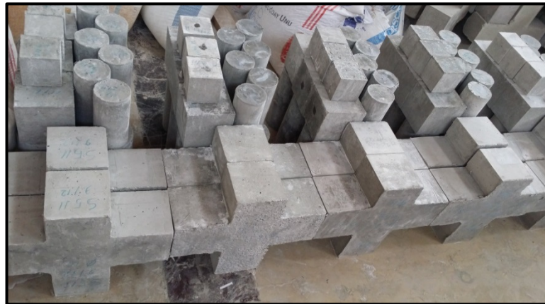
Figure 3.4 Preparing the specimens after curing treatment.
