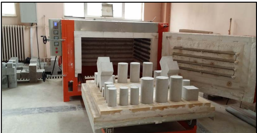
Figure 3.6 Arrangement the specimens inside the electric furnace.
