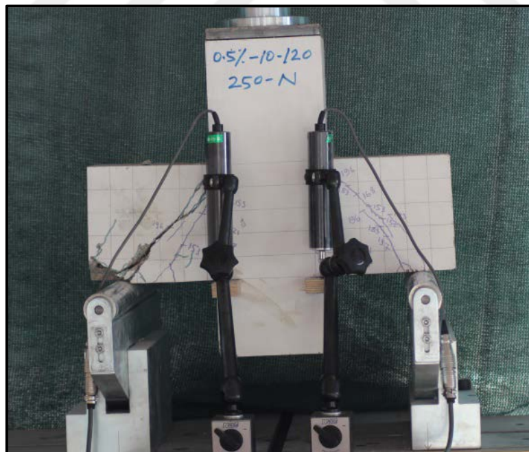
b) Adjusting the LVDT during the testing
