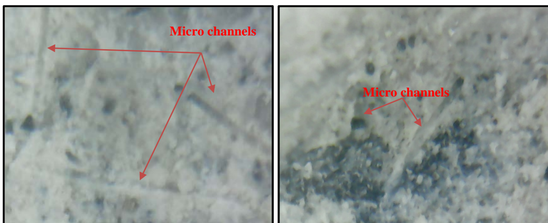
Figure 4.6 Micro channels formed by melting of PP fibers.
