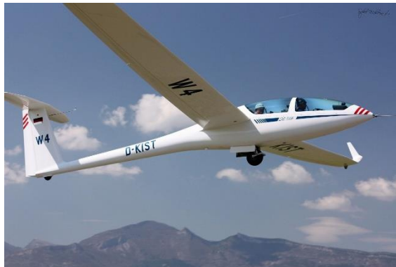
Figure 3.7 Single main landing gear configuration sailplane DG-1001T [52]
