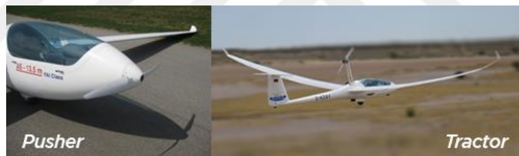
Figure 3.11 Sailplane propulsion system configurations [55,56]
