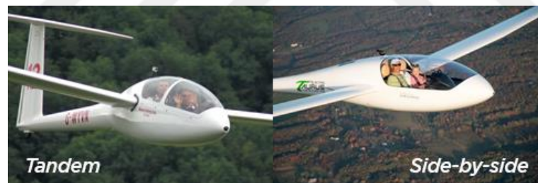
Figure 3.10 Two-seater sailplane seating configurations [53,54]
