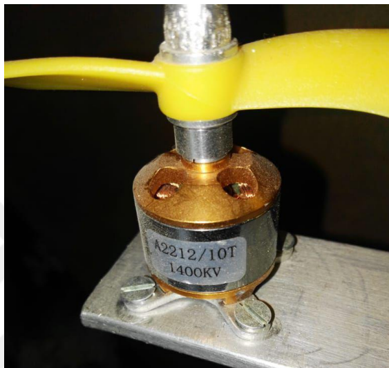
Figure 3.2 UAV Brushless Motor A2212/10 1400KV
