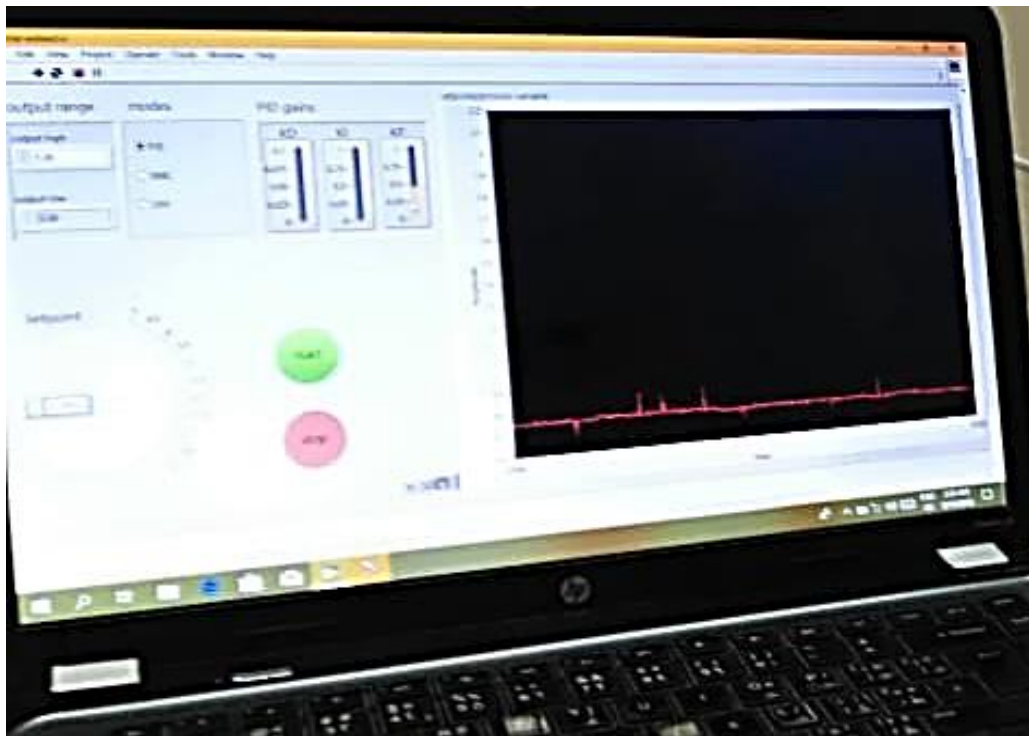
Figure 4.1 The mode selection and real-time monitoring from GUI for proposed 1-DOF helicopter
