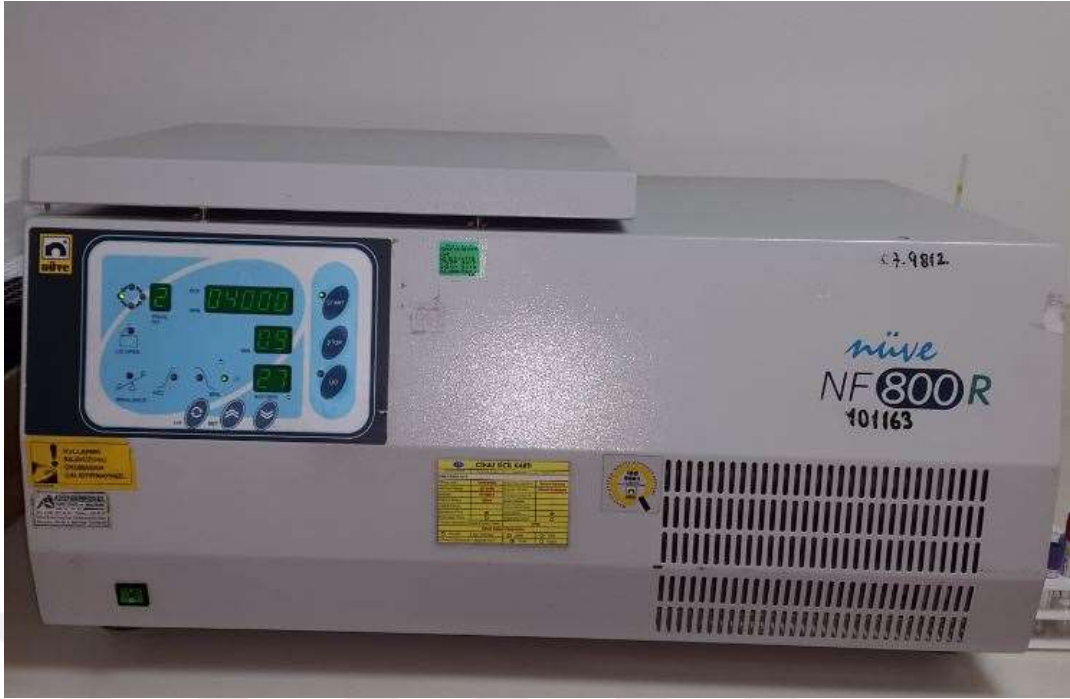
Figure 3.3 Illustrated Centrifuge instrument (Nuve NF800R, Ankara, Turkey).
