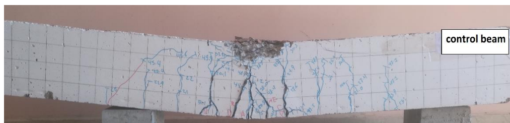
Figure 4.9 Crack pattern and failure mode of CB
