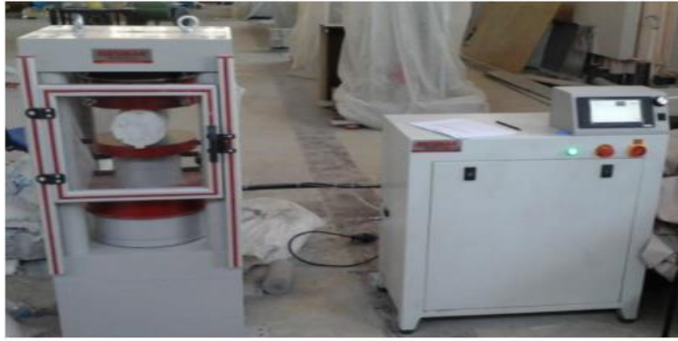
Figure 3. 12 Compressive machine test for split tensile strength test
