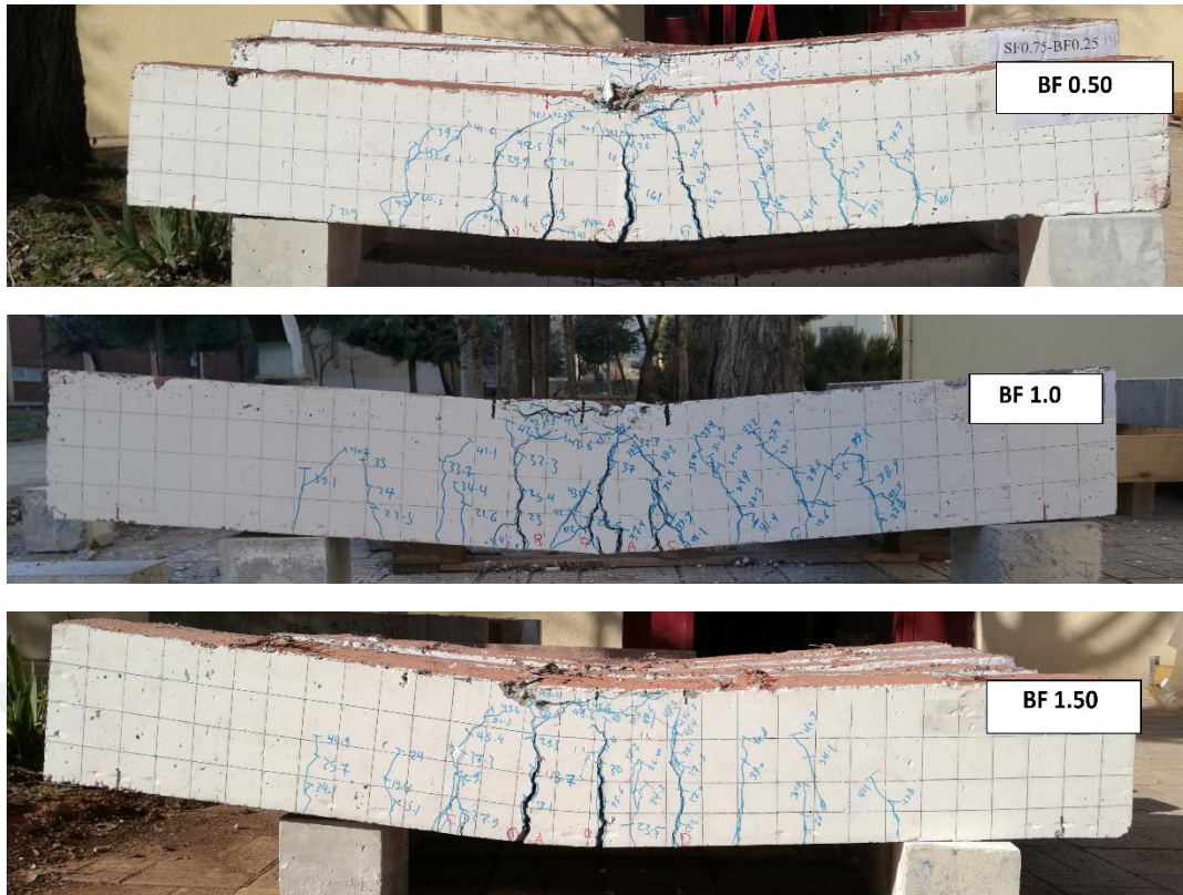
Figure 4.10 Crack pattern and failure mode of tested beams for Group (A)
