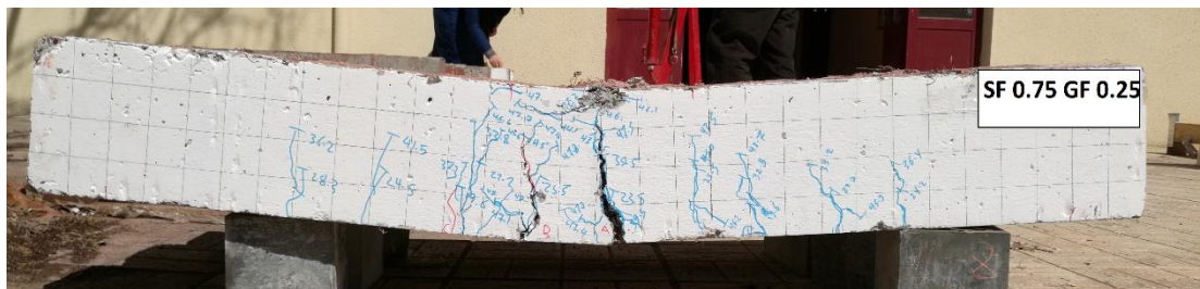
Figure 4.13 Crack pattern and failure mode of tested beams for Group (D)
