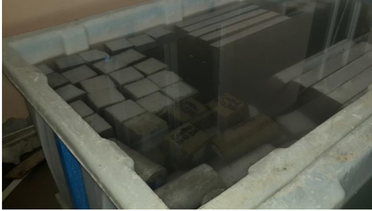
Figure 3.10 Pool curing for cube and cylinder
