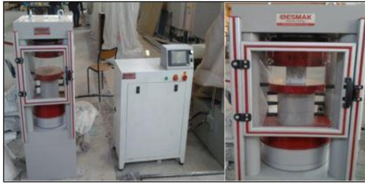
Figure 3.11 Compressive machine test for compressive strength test
