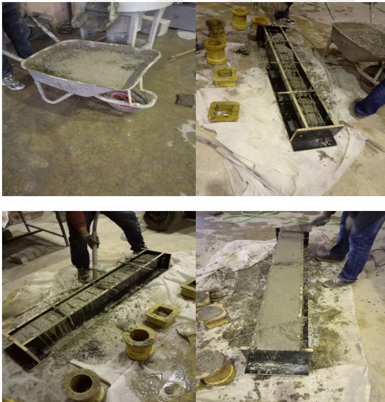
Figure 3.7 Preparing and casting of the beam specimens
