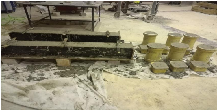
Figure 3.8 Preparing and casting of cubes and cylinders
