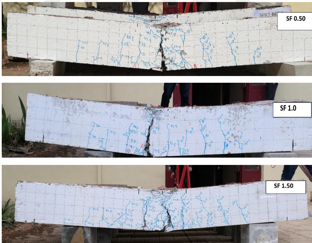
Figure 4.11 Crack pattern and failure mode of tested beams for Group (B)
