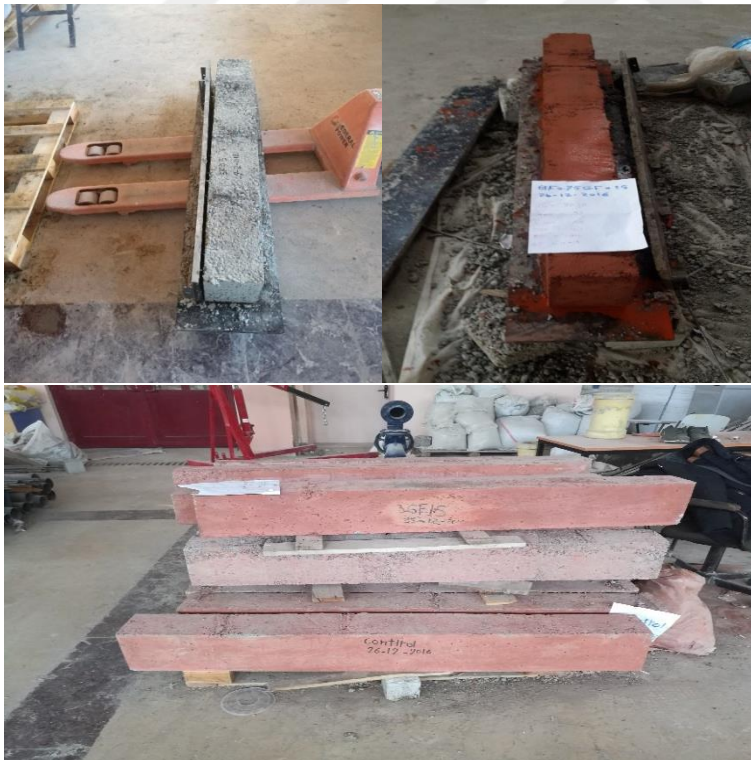
Figure 3.9 Curing of beam specimen
