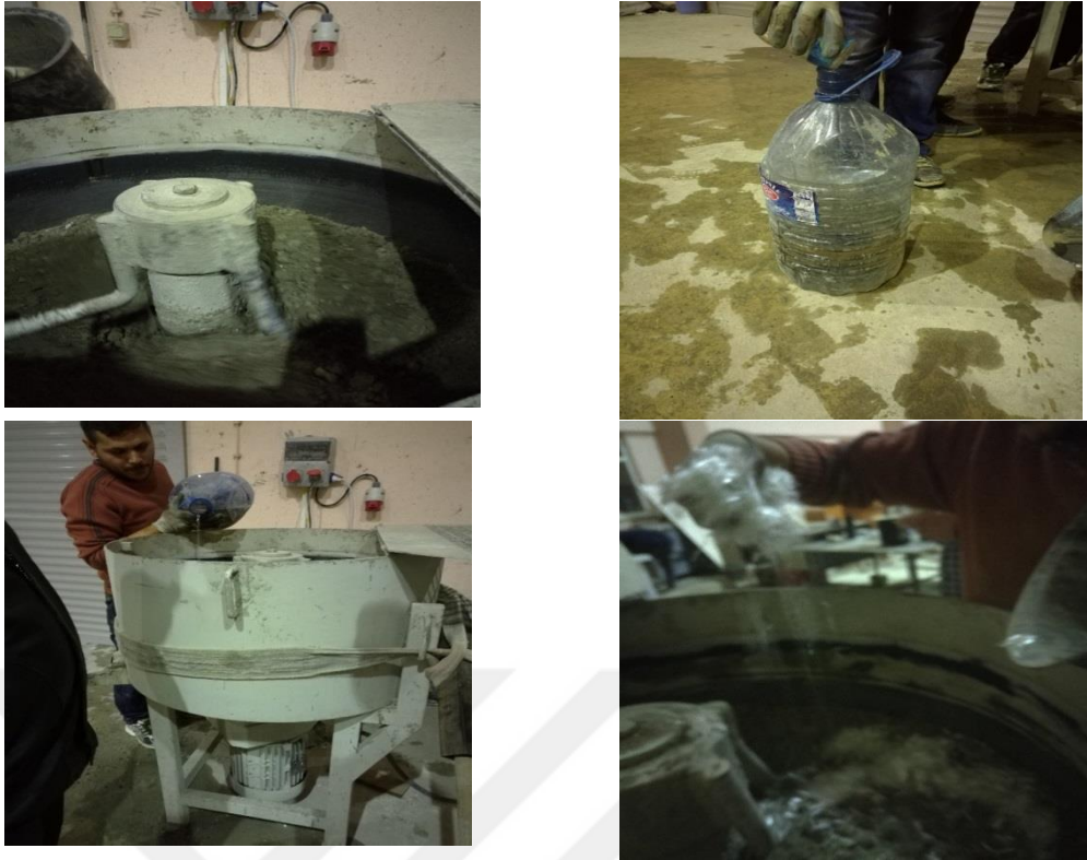
Figure 3.6 Proportioning and mixing of the specimen
