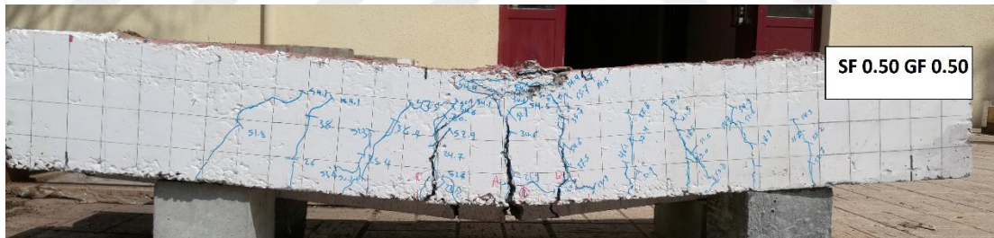
Figure 4.12 Crack pattern and failure mode of tested beams for Group (C)
