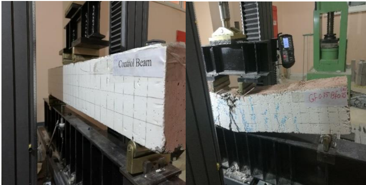
Figure 3.13 Flexural strength test machine for beam and beam failure
