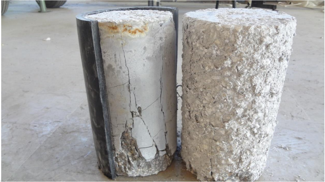
Figure (B21) HDPE tube (HSCC-G1-1%-A) and (USCC-G1-1%-A) after test
