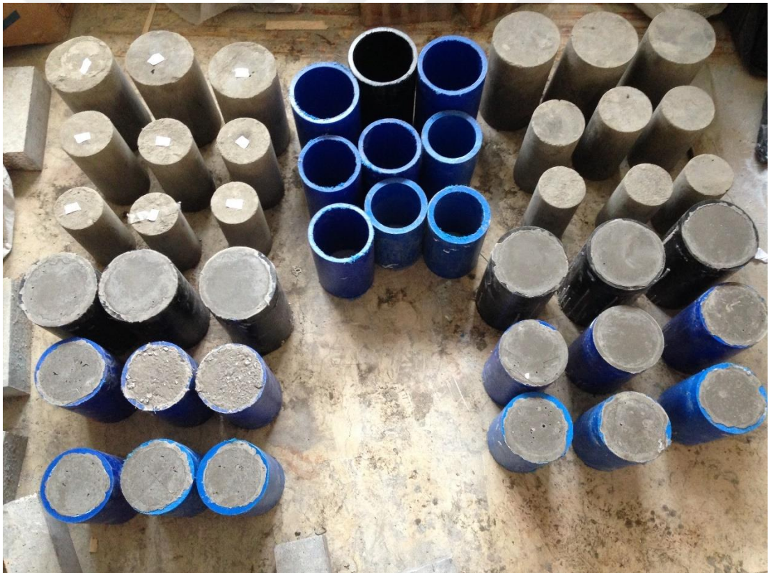
Figure (B4) HDPE tubes after the casting
