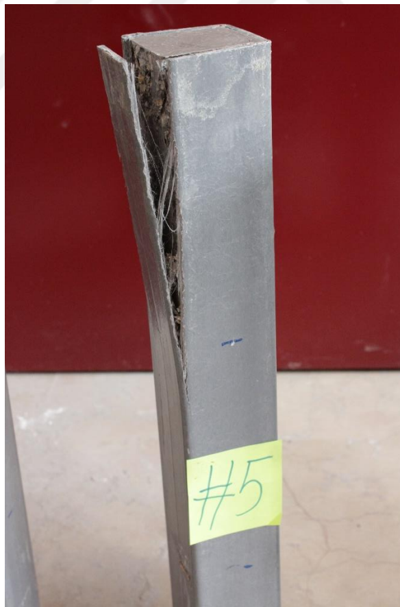
Figure (A28) GRP tube (GC-SCC-G3-0%-W) after test
