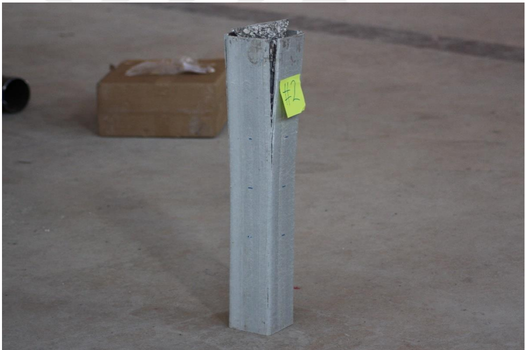
Figure (A12) GRP tube (GC-SCC-G1-1%-W) after test
