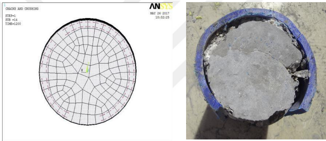
Figure (B24) Perimeter crush of concrete, ANSYS and Experimental sample
