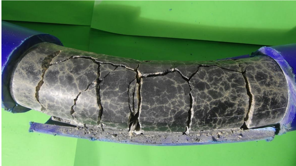
Figure 4.3 (c2) Composite beams HDPE-8 after remove the shell of HDPE tube
