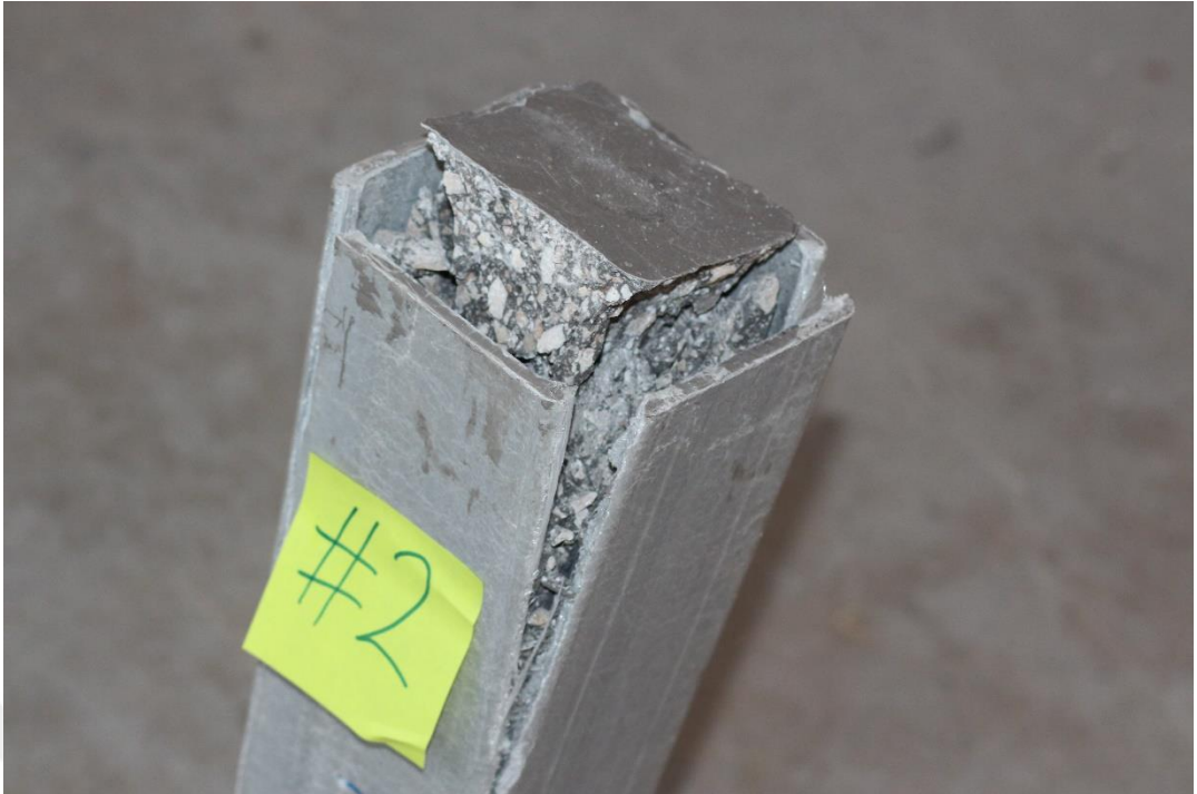
Figure (A11) GRP tube (GC-SCC-G1-1%-W) after test
