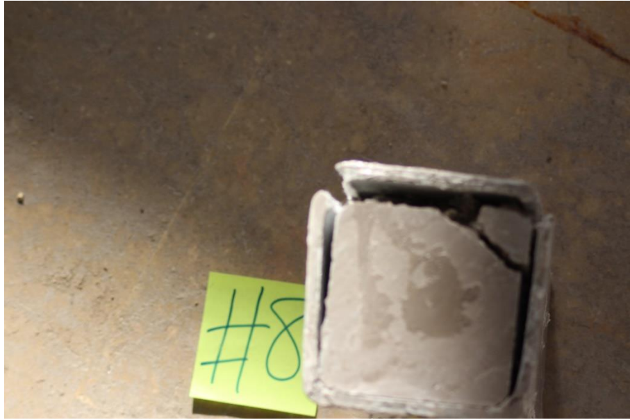
Figure (A21) GRP tube (GC-SCC-G2-1%-W) after test
