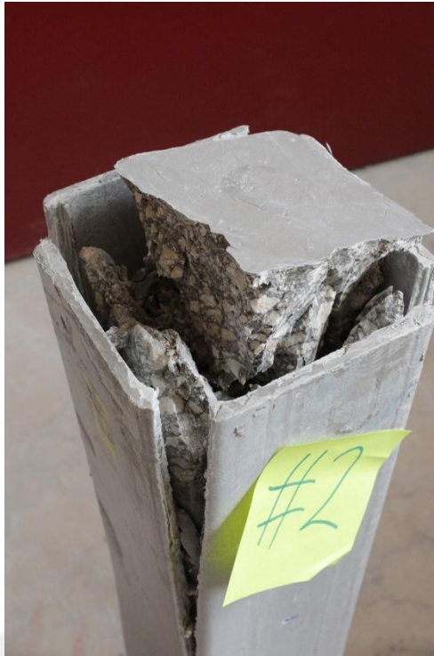
Figure (A33) GRP tube (GC-SCC-G1-1%-W) after test
