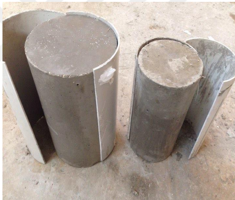
Figure 3.1 (c) Removal of formworks after hardening of SCC for unconfined specimens
