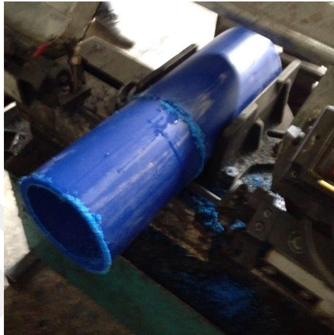
Figure (B1) first step of cutting HDPE tubes
