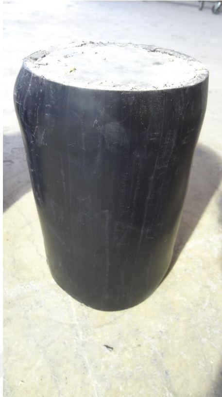
Figure (B19) HDPE tube (HSCC-G1-1%-A) after test
