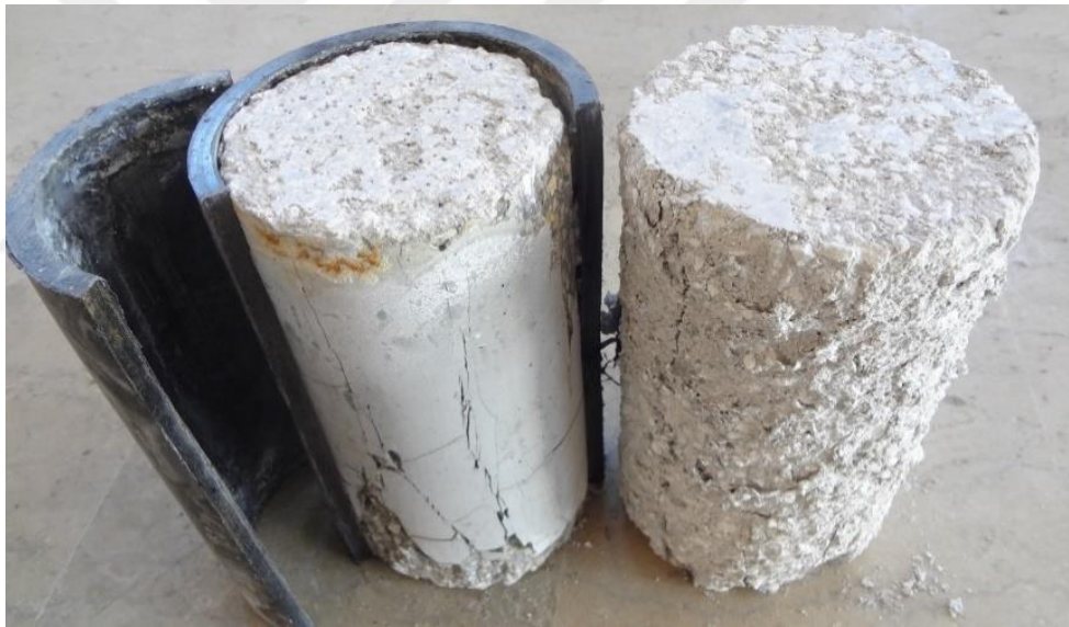
Figure 3.10 Confined and unconfined specimens after exposure to acid environment
