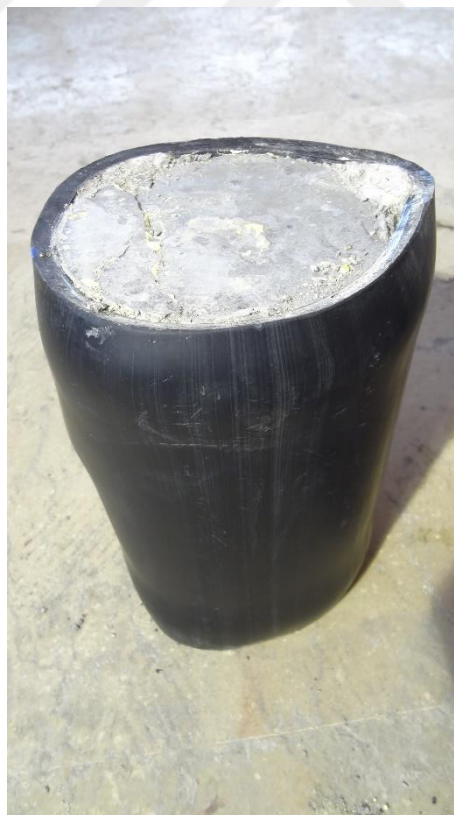
Figure (B14) HDPE tube (HSCC-G1-1%-S) after test
