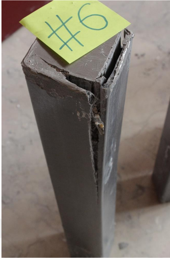
Figure (A31) GRP tube (GC-SCC-G3-1%-W) after test
