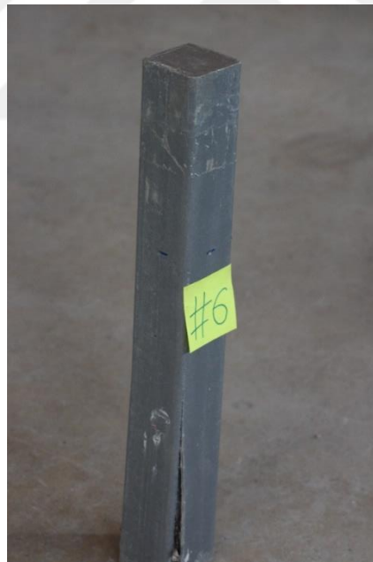
Figure (A16) GRP tube (GC-SCC-G3-1%-W) after test
