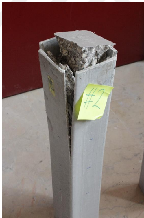
Figure (A34) GRP tube (GC-SCC-G1-1%-W) after test
