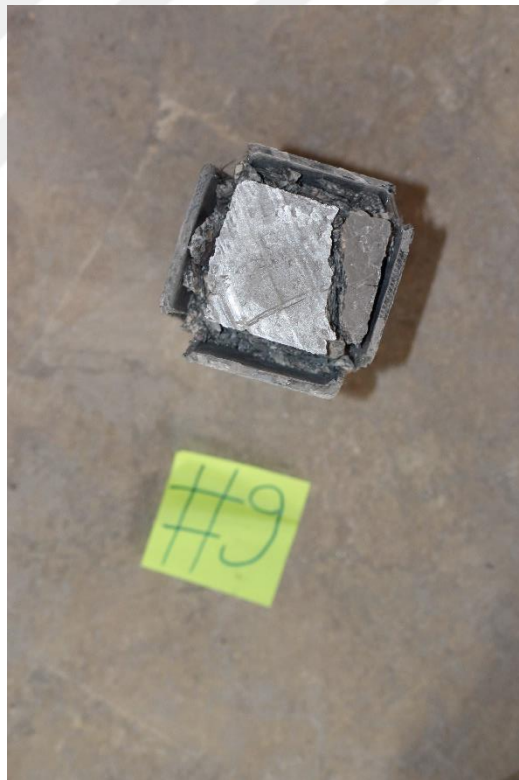
Figure (A24) GRP tube (GC-SCC-G4-0%-W) after test
