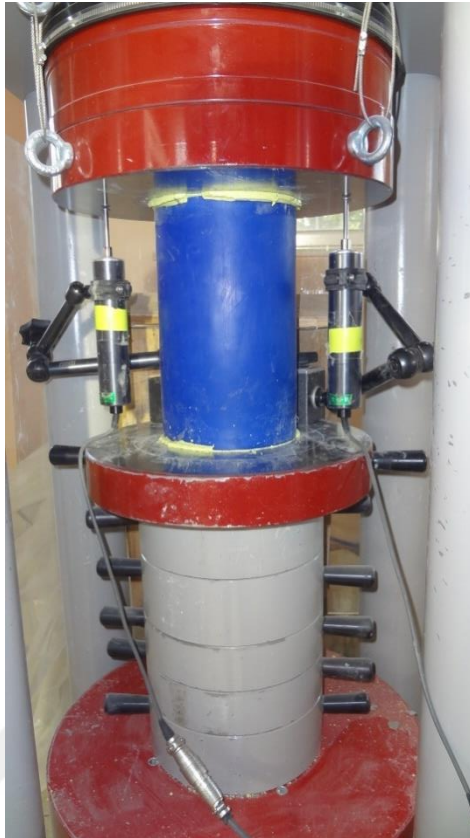
Figure (B15) HDPE tube (HSCC-G2-0%-W) step 1 for the test
