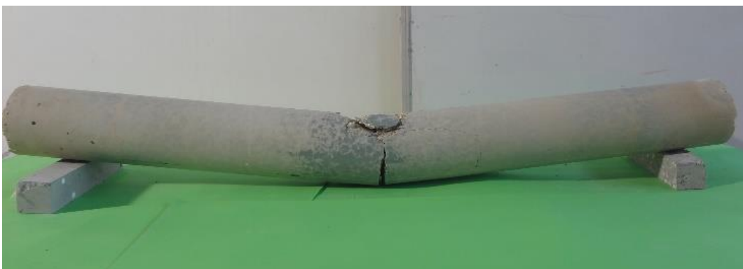
Figure 4.3 (d) Composite beams SCGP -14 after tested
