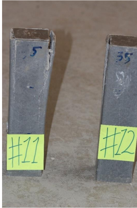
Figure (A25) GRP tube (GC-SCC-G4-1%-A) and (GC-SCC-G4-0%-A) after test
