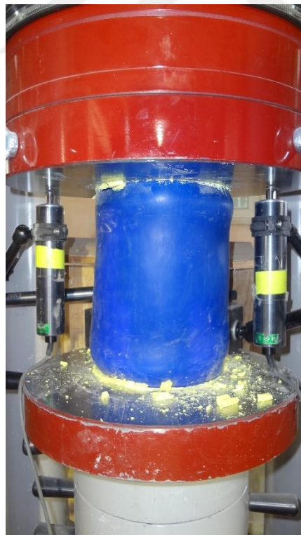
Figure (B16) HDPE tube (HSCC-G2-0%-W) step 2 for the test
