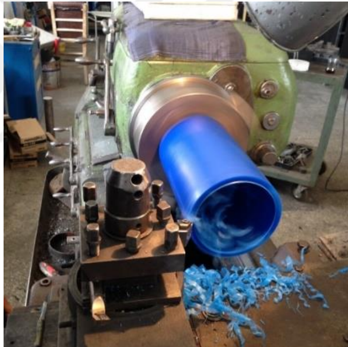
Figure 3.1 (a) Cutting of HDPE tube
