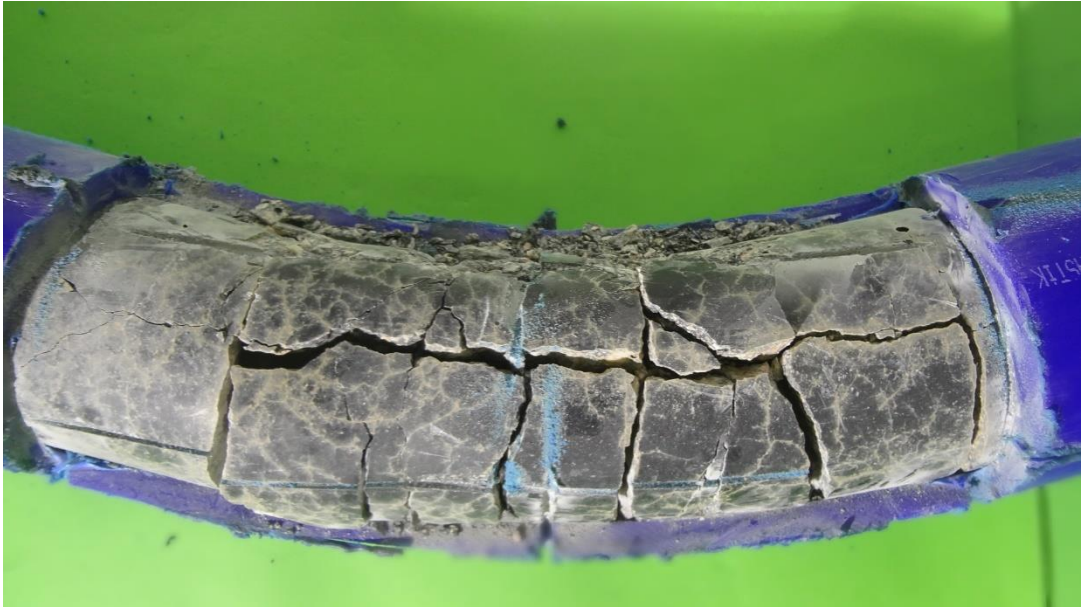
Figure 4.3 (b2) Composite beams HDPE-10 after remove the shell of HDPE tube
