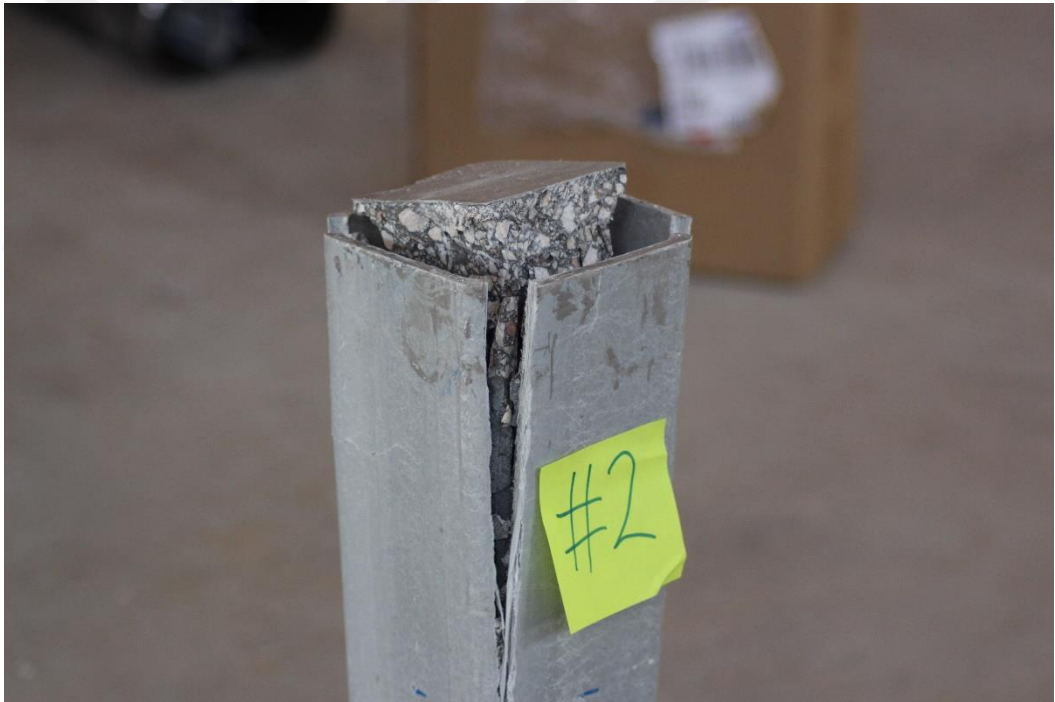
Figure (A10) GRP tube (GC-SCC-G1-1%-W) after test
