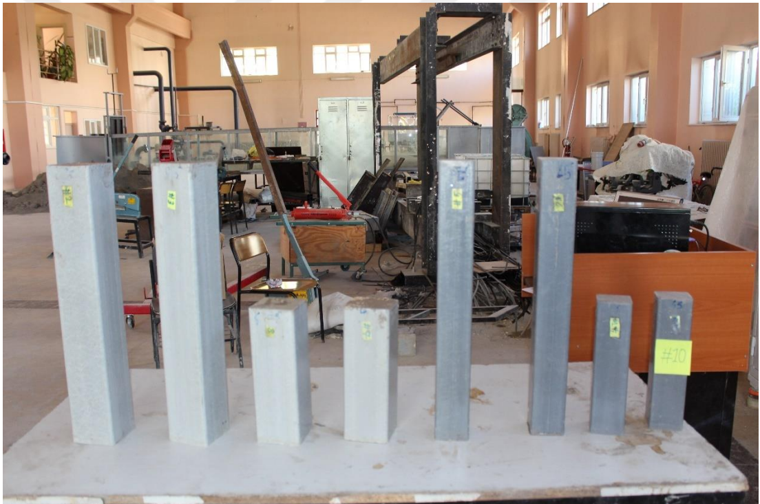
Figure (A4) GRP tube prepare to test
