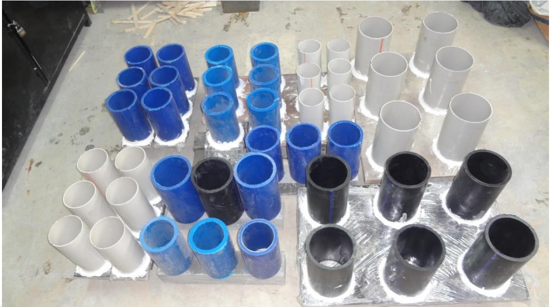
Figure (B3) HDPE tubes before the casting
