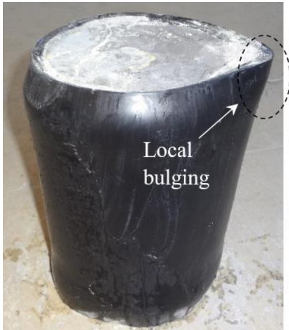
Figure 3.4 (a) Shear type failure (HSCC)
