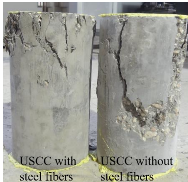
Figure 3.4 (c) Failure types of USCC specimens
