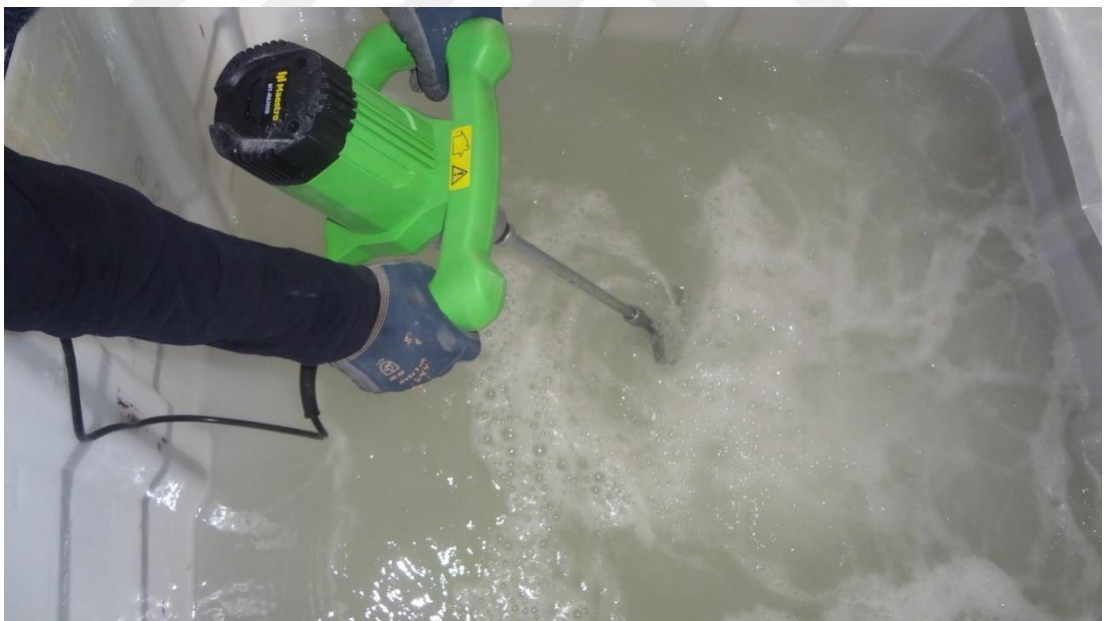
Figure (B6) The acid and sulfate solution were prepared mechanically to insure the uniform concentration of particles in solution
