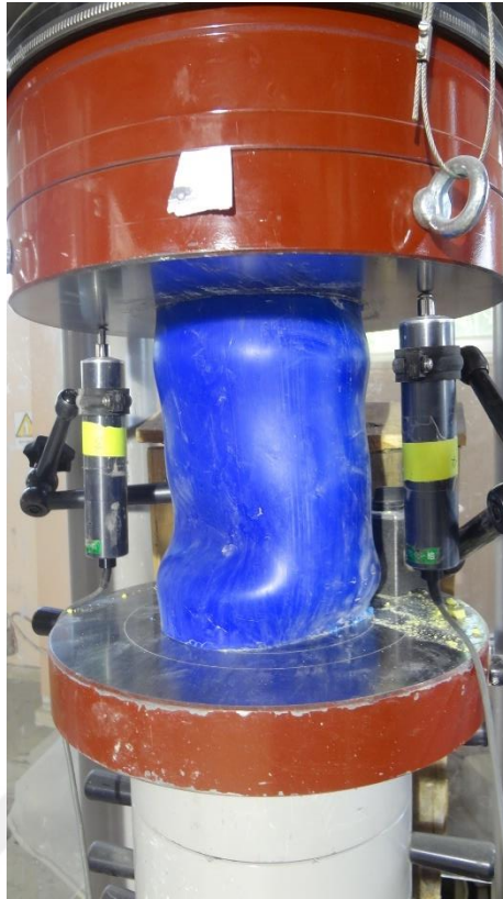
Figure (B9) HDPE tube (H-G1-W) step 3 for the test
