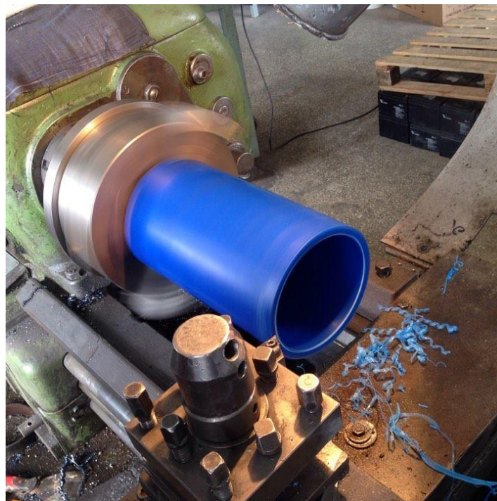
Figure (B2) second step of cutting HDPE tubes
