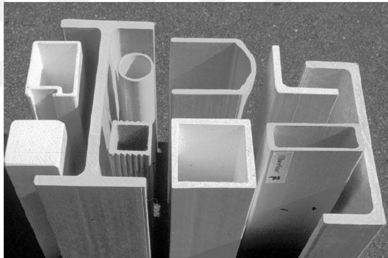
Figure 1.1 FRP profiles of various cross-section shapes (Zhao, 2017)
