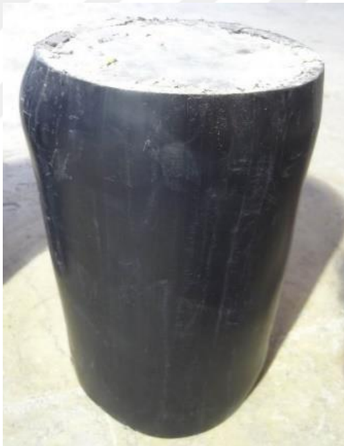
Figure 3.4 (b) Drum type failure (HSCC)
