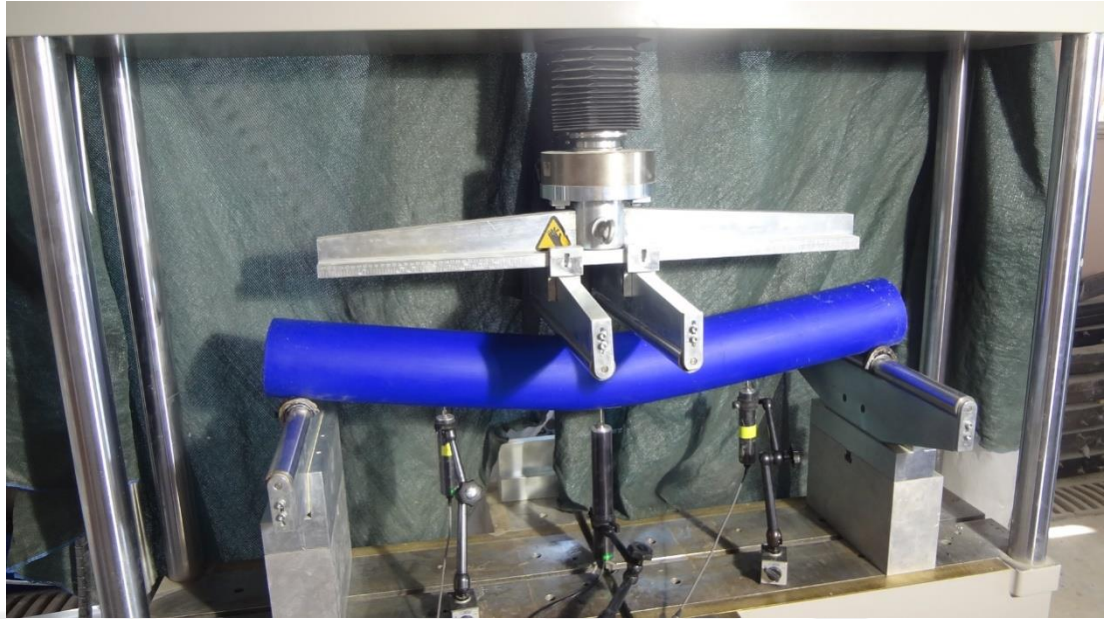
Figure (C9) HDPE-2 step 2 for the test
