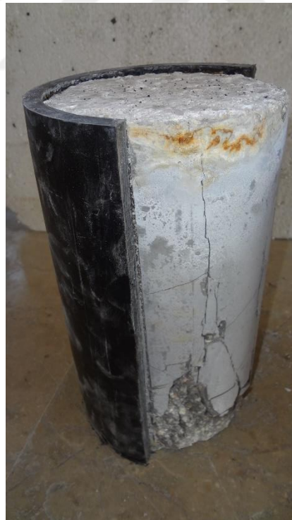
Figure (B20) HDPE tube (HSCC-G1-1%-A) after test
