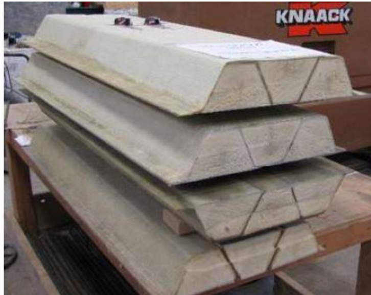
Figure 1.4 FRP panels filled with foam material (Zhao, 2017)
