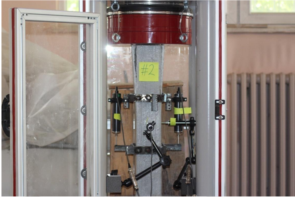
Figure (A9) GRP tube (GC-SCC-G1-0%-W) after test
