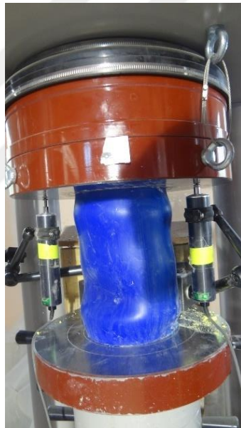
Figure (B8) HDPE tube (H-G1-W) step 2 for the test
