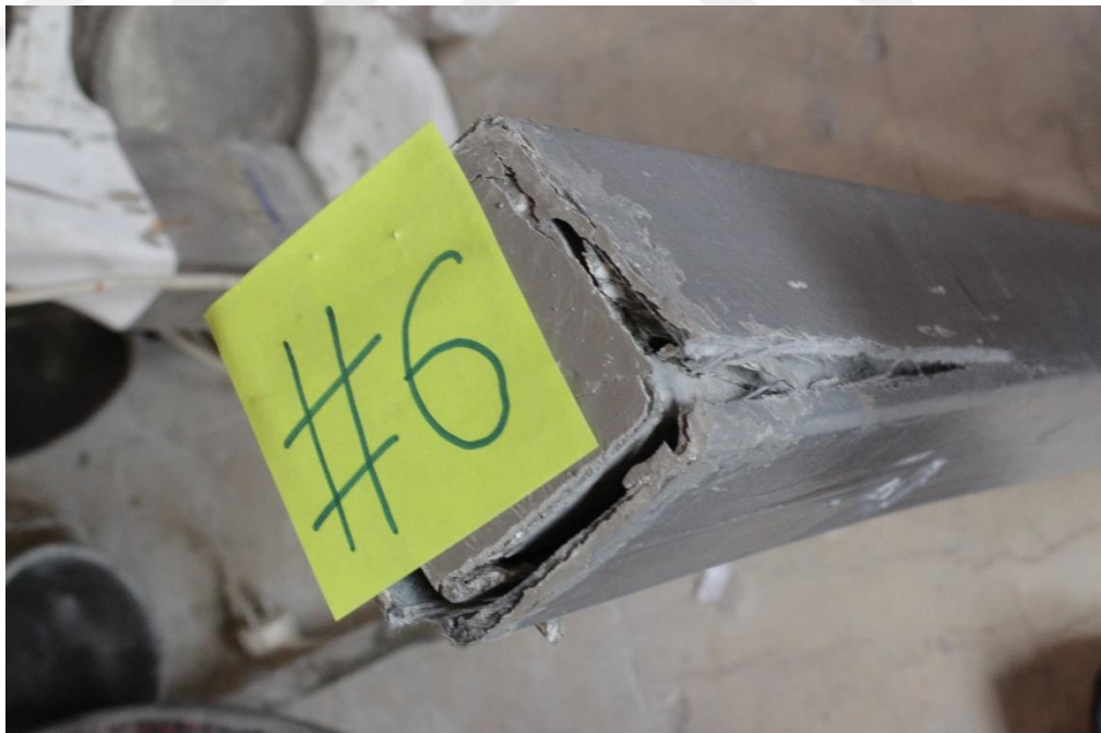
Figure (A32) GRP tube (GC-SCC-G3-1%-W) after test
