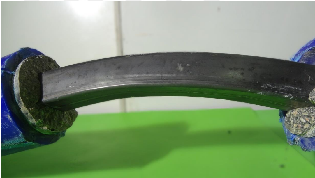
Figure 4.3 (b3) Composite beams HDPE-10 after remove the SCGP
