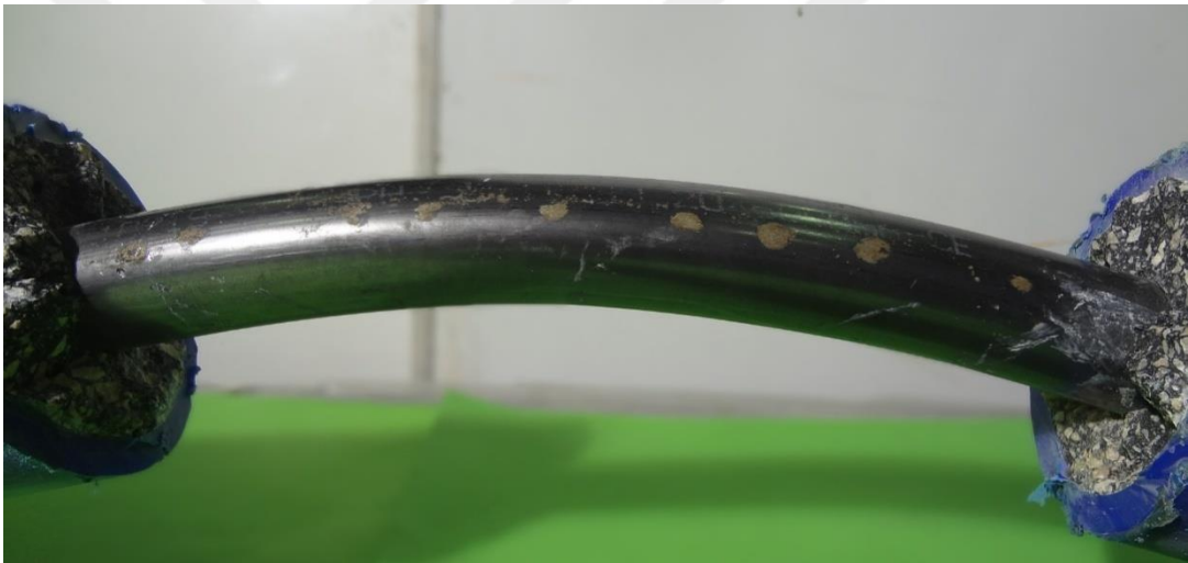
Figure 4.3 (c3) Composite beams HDPE-8 after remove the SCGP
