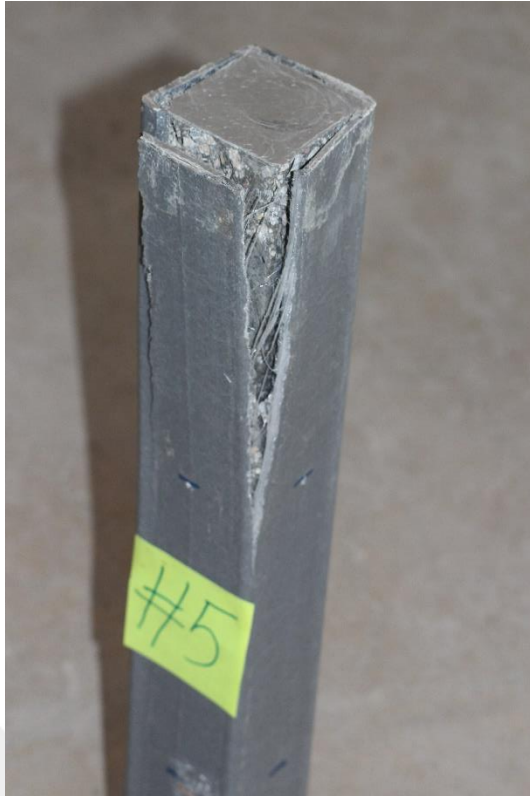
Figure (A15) GRP tube (GC-SCC-G3-0%-W) after test
