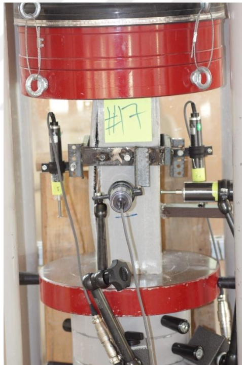
Figure (A26) GRP tube (GC-SCC-G2-1%-W) during test
