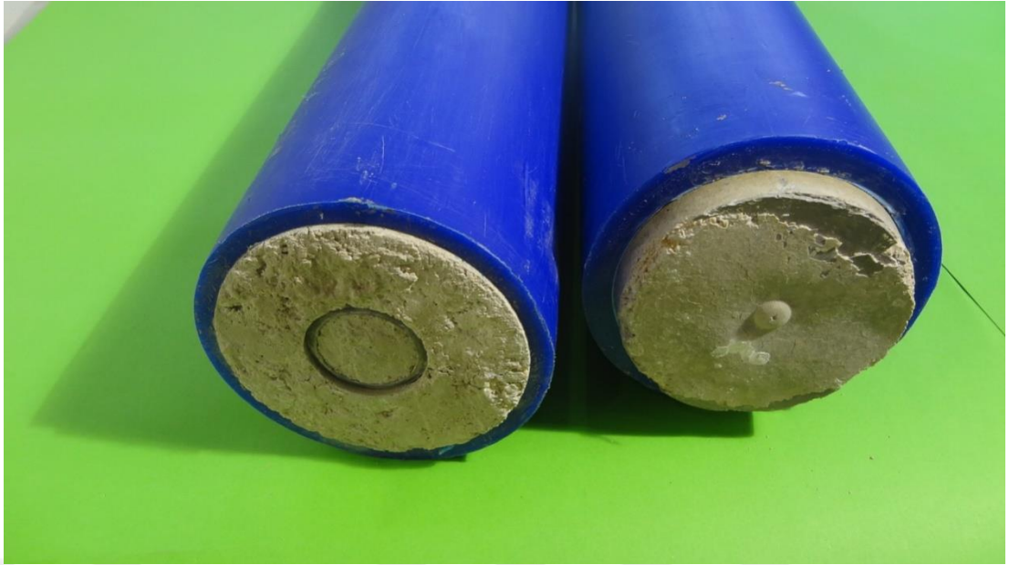
Figure (C21) HDPE-7 and HDPE-11 after the test
