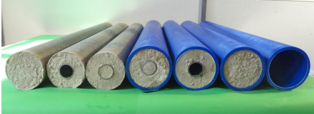
Figure 4.2 (e) Specimens after SCGP pouring
