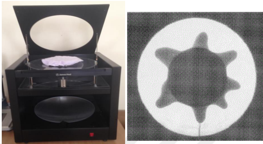
Figure 3.44 a)Drapeability tester; b) Shadow of fabric tested
