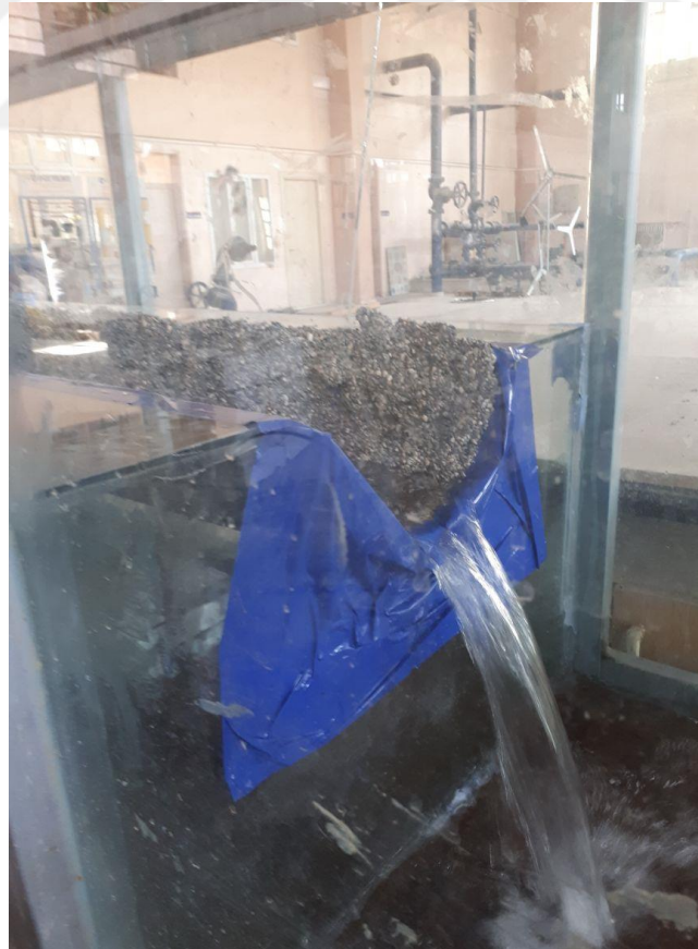
Figure 4.11 Free Overfall in Semicircular Channels with (2 mm) Roughness on Bottom
