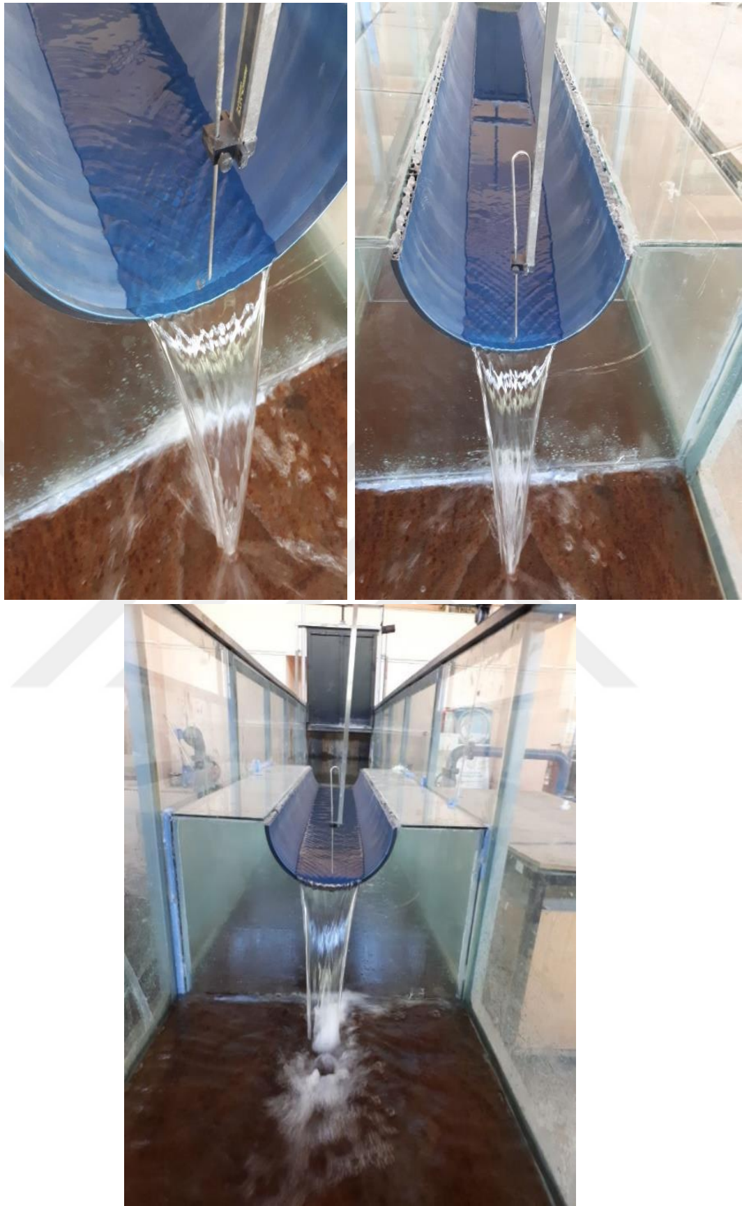
Figure 4.10 Free Overfall in Semicircular Channels with Smooth Bottom
