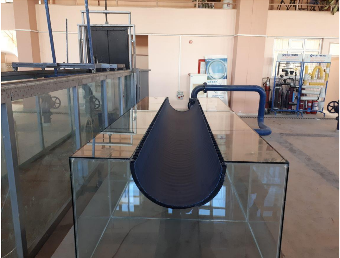
Figure 4.9 (c) Semicircular Channel (View 1)
