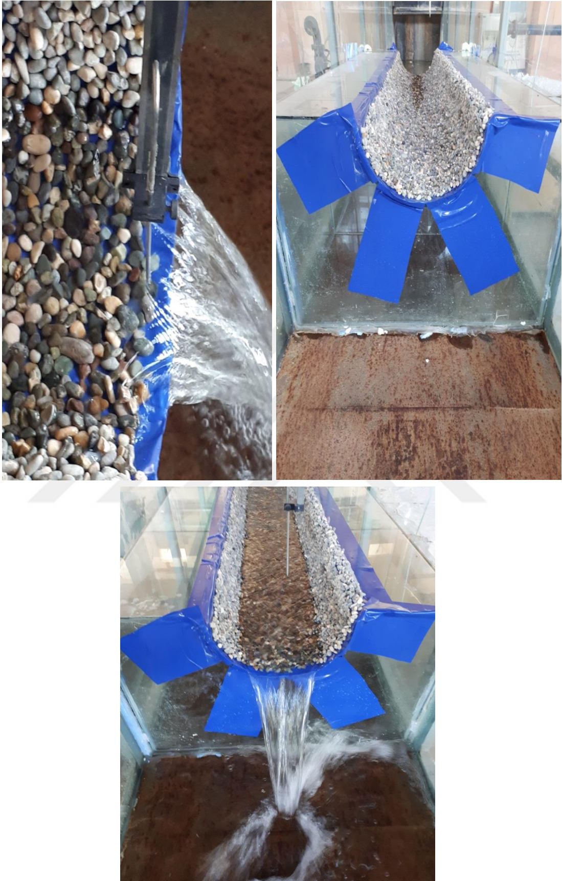
Figure 4.13 Free Overfall in Semicircular Channels with (6.33 mm) Roughness on Bottom
