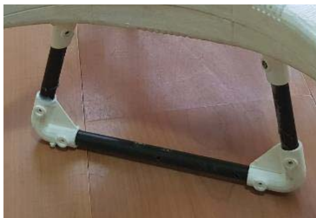
Figure 6.16 Landing Gear Assembly
