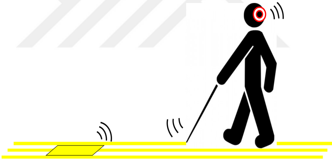
Figure 1.1 View of the knowledge transmitter unit embedded into the tactile pathway having embossed straight lines.
