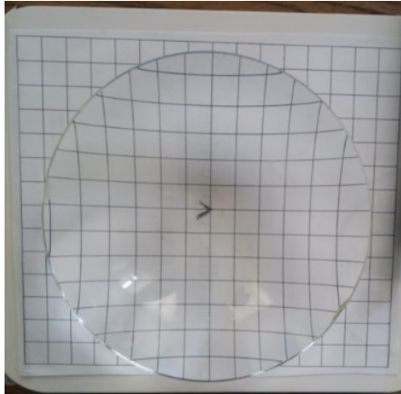
Figure 2.19 Pincushion distortion aberration
