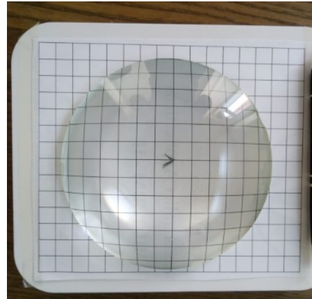
Figure 2.20 Barrel distortion aberration
