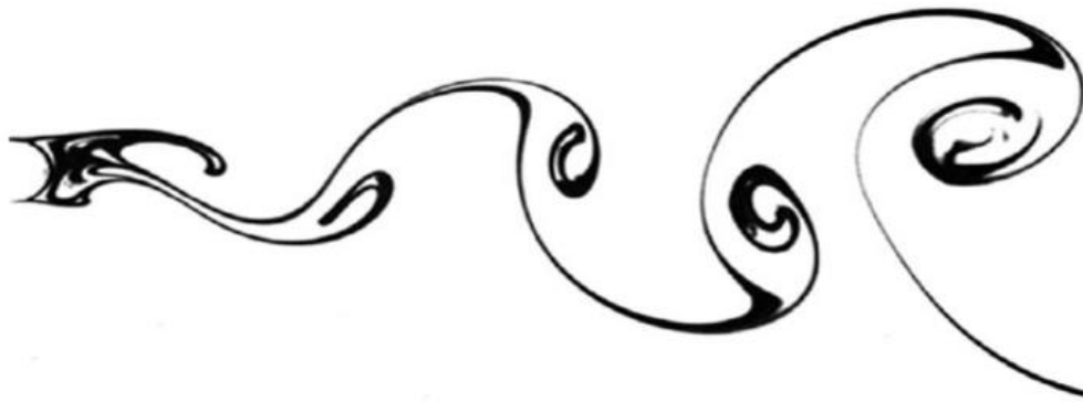
Figure 2.1 Vortex shedding in the wake region of the flow past a circular cylinder (Dyke, 1982)
